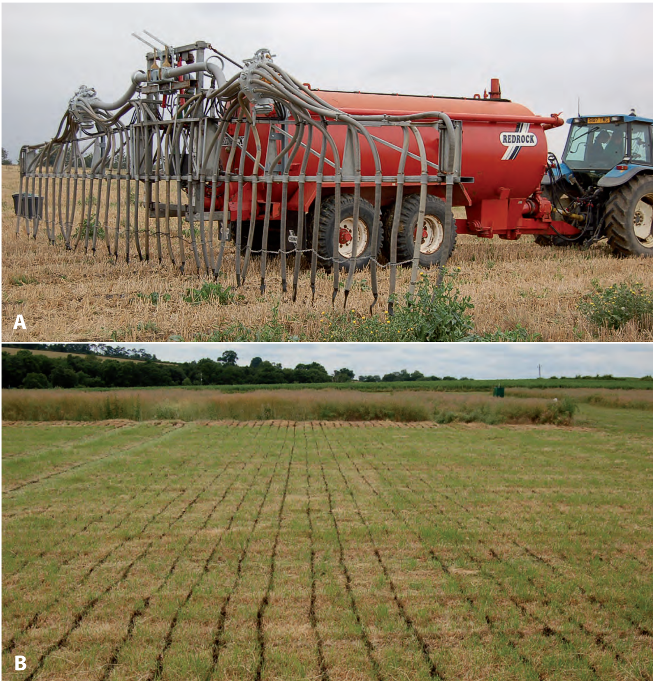
Image 17: Trailing-hose band-spreader (A) (Field Measure 6). By setting the exit pipes immediately above the ground and by correct dosing, the result should achieve narrow bands of slurry on the surface (B), which reduce ammonia emissions while aiding infiltration (photographs: © ADAS).
