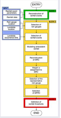
**Figure C2** Logical framework of the algorithm in CTRL-T.
