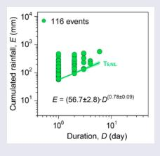
**Figure C6** *ED* rainfall conditions that have produced landslides in Nilgiris Pilot area (116 green dots). Green curve is 5% power law threshold for Nilgiris (T5,NIL). The shaded area shows the uncertainty associated with the threshold curve. Data are in logarithmic coordinates.
