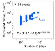
**Figure C4** *ED* rainfall conditions that have produced landslides in Darjeeling pilot area (84 blue dots). Blue curve is 5% power law threshold for Darjeeling (T5,DAR). The shaded area shows the uncertainty associated with the threshold curve. Data are in logarithmic coordinates.
