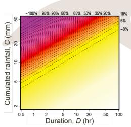
**Figure A3** Graphical representation of the short-range landslide probabilistic forecast model. The model associates any *C* vs *D* rainfall condition measured or forecasted in an area, to a correspondent Non Exceedance Probability (NEP) value expressed in %.
