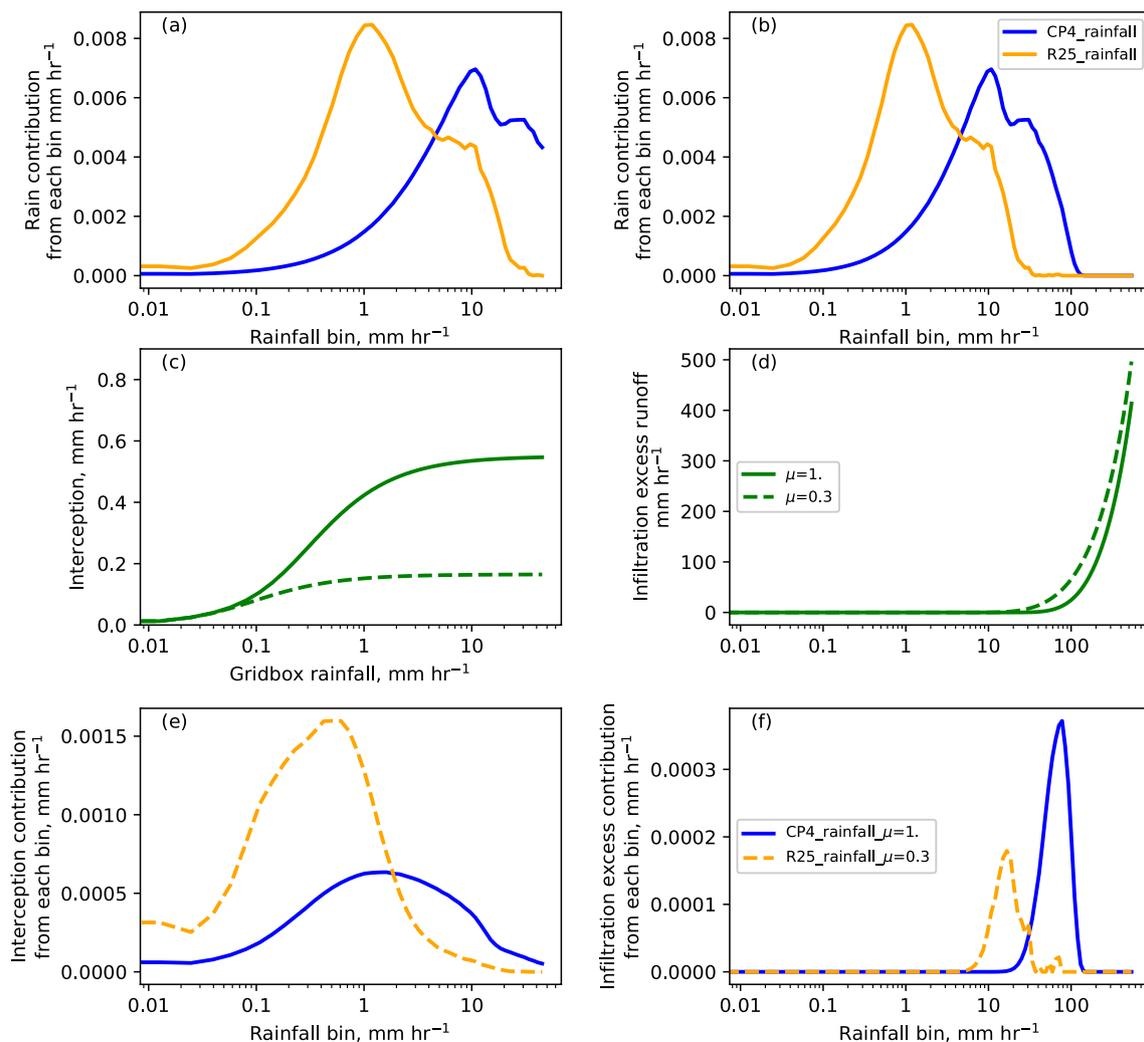
**Fig. 2** **a** and **b** show the contribution of hourly rainfall in CP4 (blue) and R25 (orange) to average grid box rainfall over a Central Africa sub-region (27.8–28.8° E, 4.5–5.5° N). The same distributions are shown on **a** and **b** but the x-axis range is reduced for (a, c and e). The sub-grid rainfall relationships from Eqs. 2 and 3 for **c** interception and **d** infiltration excess runoff respectively, under different assumptions
