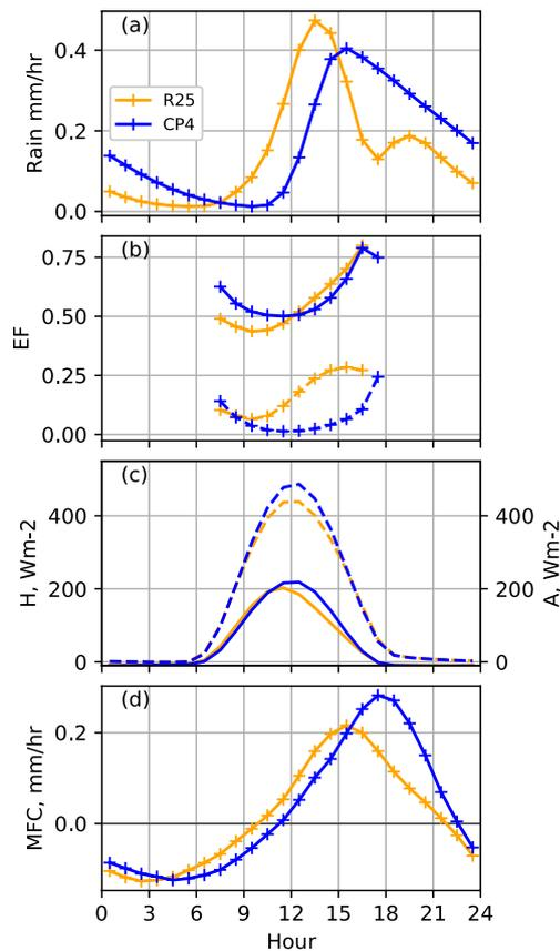
**Fig. 5** Diurnal cycles over land ( $-8$  to  $6^\circ$  E,  $5$ – $10^\circ$  N) averaged over March, April and May for **a** rainfall, **b** day time evaporative fraction (solid) and its contribution from canopy evaporation (dashed) **c** sensible heat (solid) and available energy (dashed) and **d** total column moisture flux convergence
