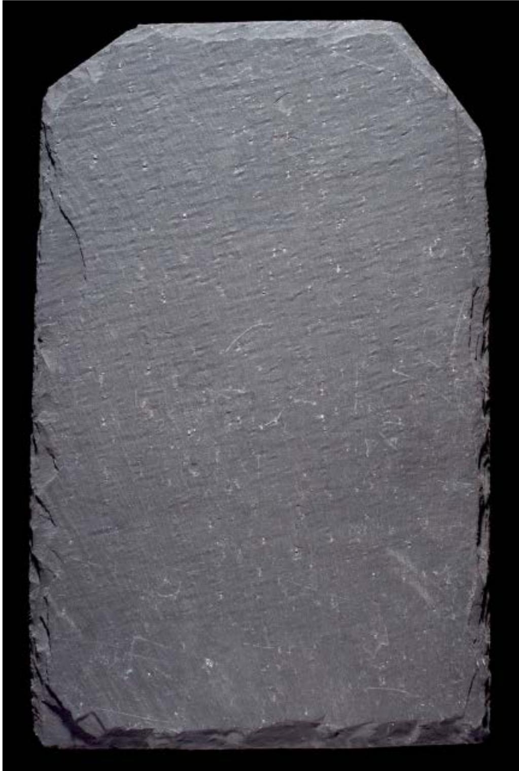
**Figure 26. A specimen of roofing slate similar to that produced in the Cullipool quarries**
