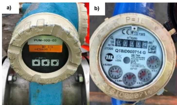
**Figure 3a) Endress + Hauser Promag flow meter. b) Maddalena DS-TRP flow meter**
