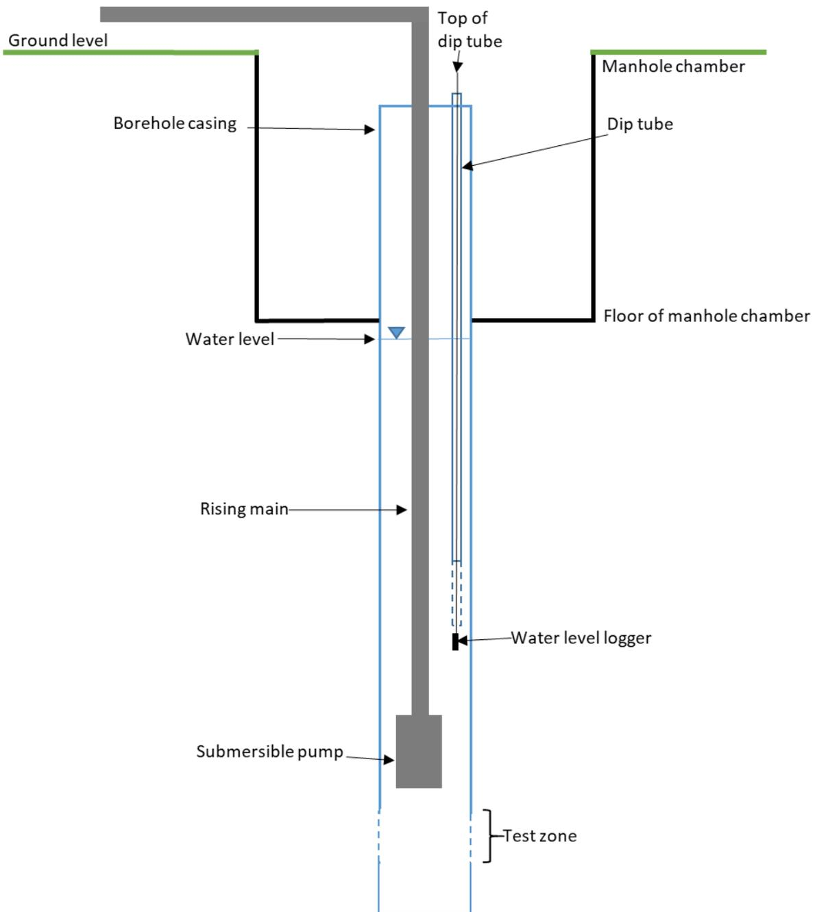
**Figure 4 Borehole design schematic including equipment used during test pumping. Made ground and superficial deposits steel casings are installed within the boreholes but not shown here for simplicity.**
