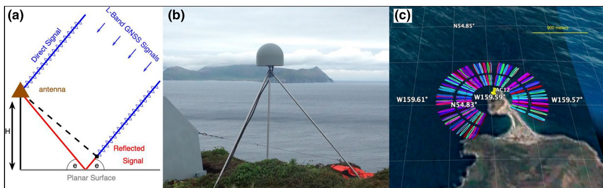
Figure 1. (a) Representation of reflected GNSS signal geometry. H is the vertical distance between the phase center of the GNSS antenna and the reflecting surface and e is the angle between the satellite and the horizon. Direct GNSS signals are shown in blue; the additional path traveled by the reflected signal is shown in red. (b) GNSS receiver AC12 on Chernabura Island, Alaska (Photo credit: UNAVCO). (c) Reflection zones shown in color were used for AC12 water level measurements (Roesler & Larson, 2018). Map courtesy of Google Earth.
