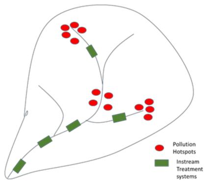
Figure 2: An example of catchment management intervention through decentralised in- drain sewage treatment
