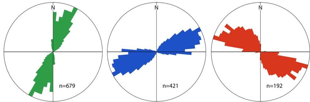
**Figure 9.** The rose diagram of the 2 m bathymetric data set can be portioned to reflect different groups of lineaments in the TAG area. Axis parallel (green, left), oblique to the axis (blue, middle), and perpendicular to the axis (red, right). These three groups represent different stress and strain regimes and tectonic processes in the evolution of the TAG hydrothermal field (5° divisions).
