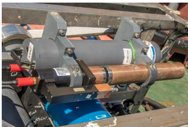
Satlantic SUNA SN 745 nitrate sensor (plastic housing, wrapped in copper tape) with integrated wiper deployed on the sensor frame
