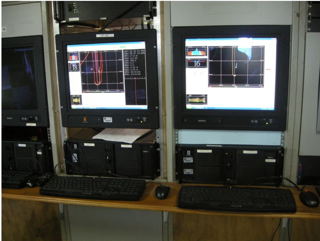
Figure 6. Acquisition set up for the EM3002 (left) on board the R/V Justo Sierra .
