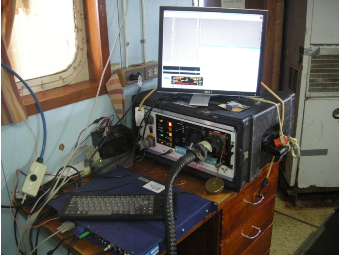
Figure 2. Acquisition set up for the CODA DA500 on board the R/V Justo Sierra .
