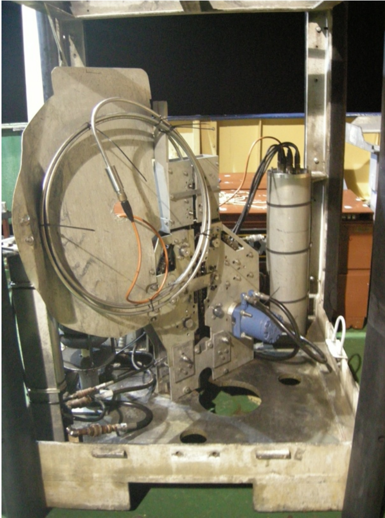
Figure 8. Detail photograph of the Seafloor Geotec CPT system used during the Yucatan 2013 cruise on board the R/V Justo Sierra .
