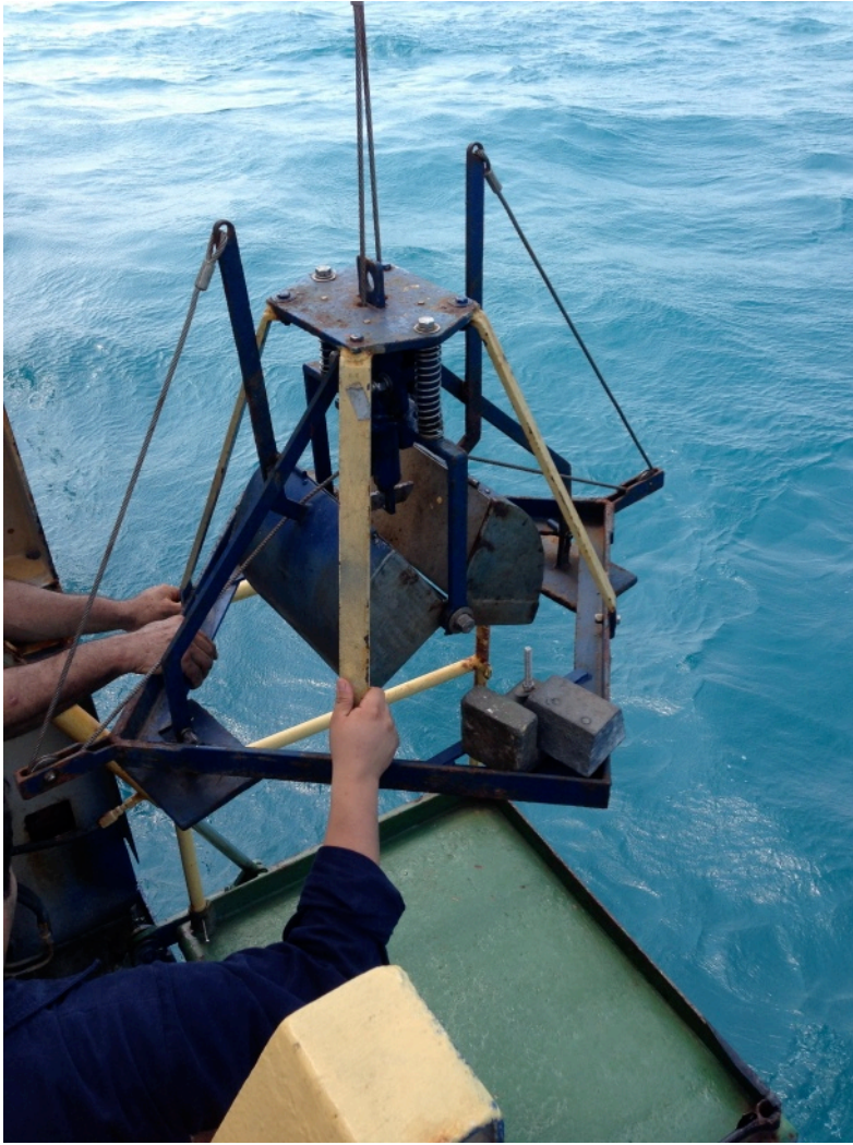
Figure 9. Photograph of the Smith-McIntyre grab being deployed from the R/V Justo Sierra .
