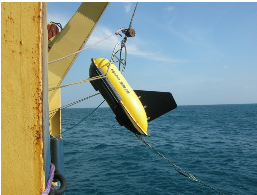
Figure 4. The EdgeTech 2000-DSS side scan sonar being deployed from the R/V Justo Sierra .
