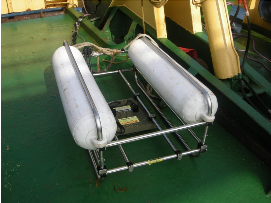
Figure 1. The Applied Acoustics surface tow boomer catamaran used during the course of this survey on the deck of the R/V Justo Sierra .
