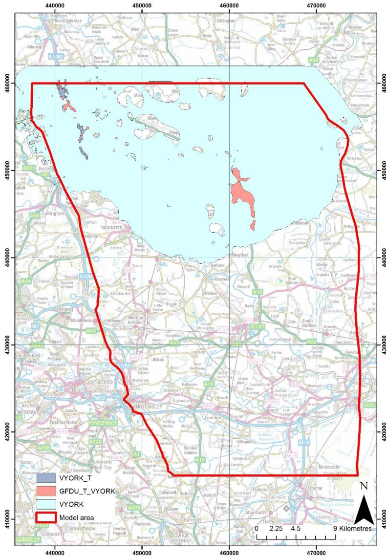
Figure 31 Distribution of the three component till units that make up the Vale of York till. © Crown copyright and database rights (2017) Ordnance Survey (100021290 EUL).
