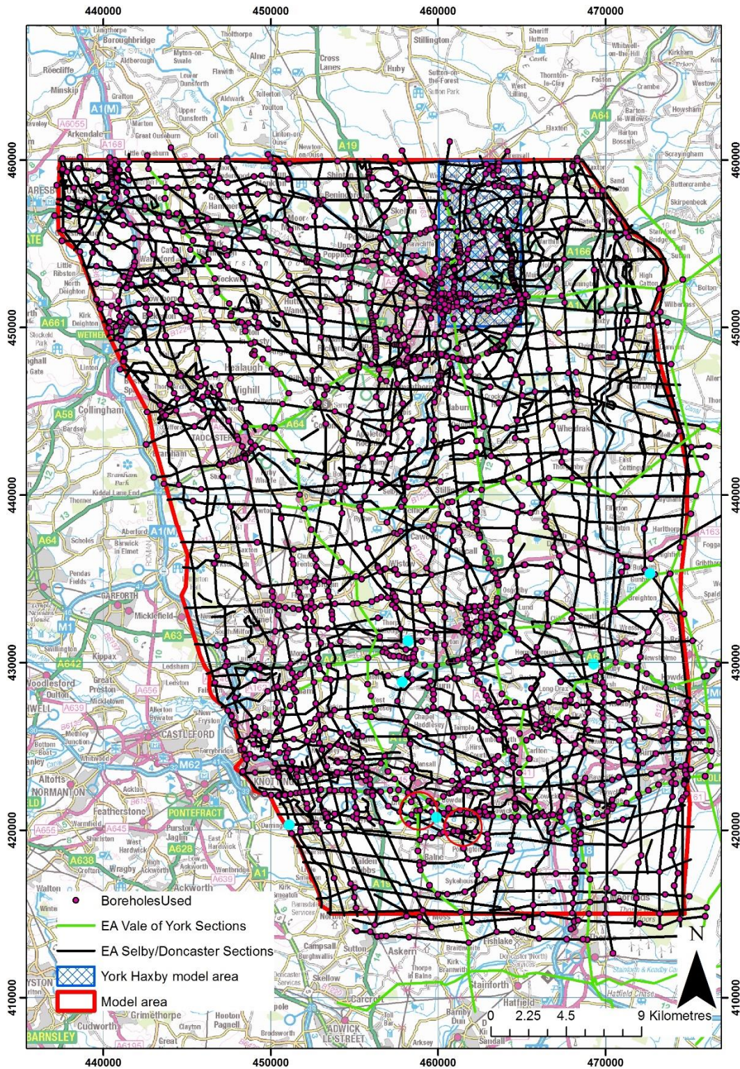
Figure 4 Distribution map of all 2,083 BGS boreholes (pink dots) and six EA boreholes (light blue dots) used to inform the 289 cross-sections that constrain the Selby model. The Heck-Pollington study area is shown as red circles. © Crown copyright and database rights (2017) Ordnance Survey (100021290 EUL).
