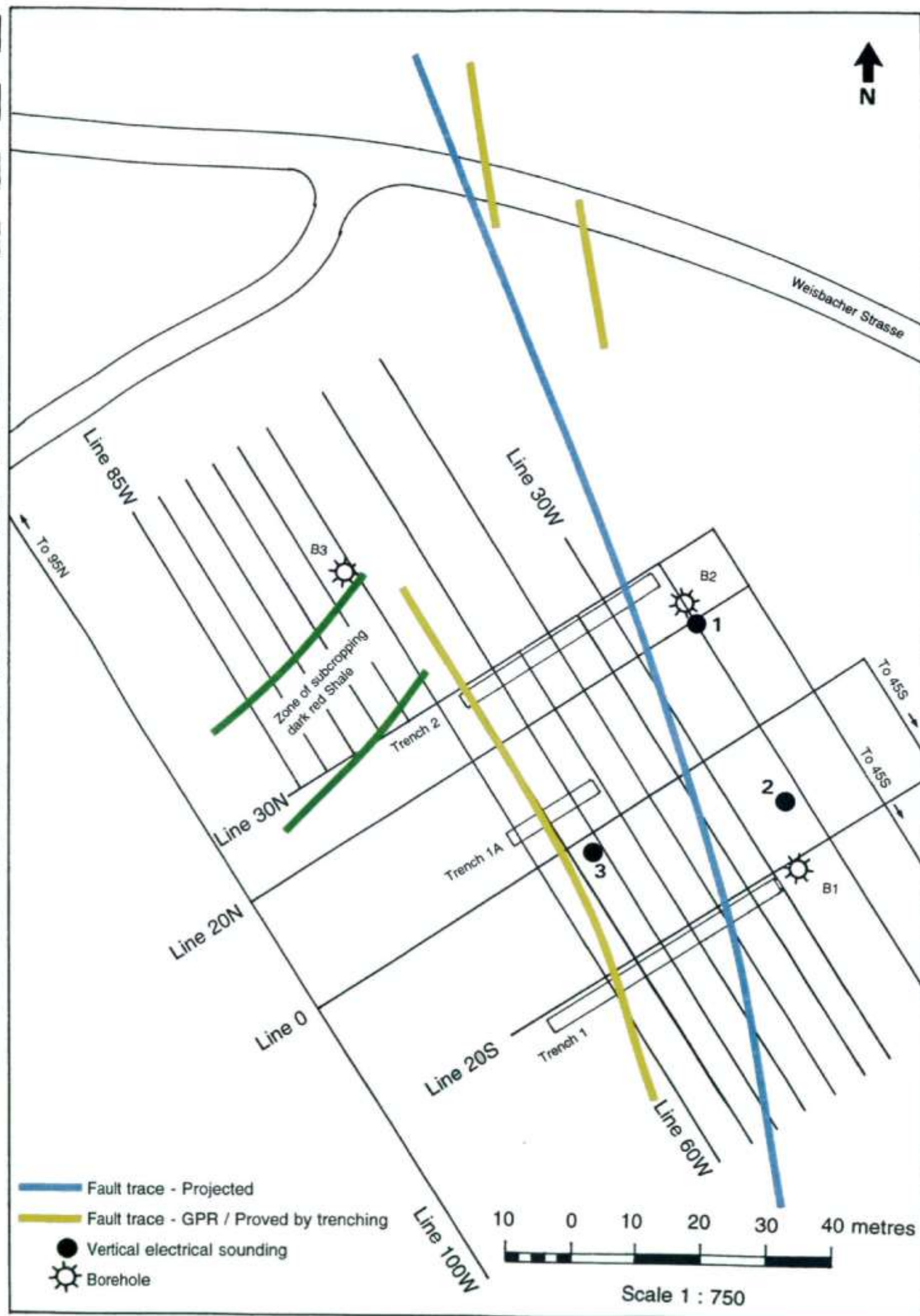
Figure 15. Test Site 2.1. Geophysical grid, trench and borehole locations, and interpretation. May 1992 survey.
