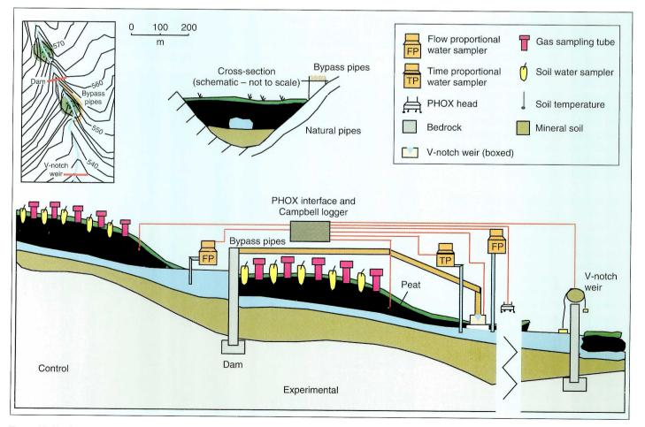
Figure 44. Design and instrumentation of the experimental field site
