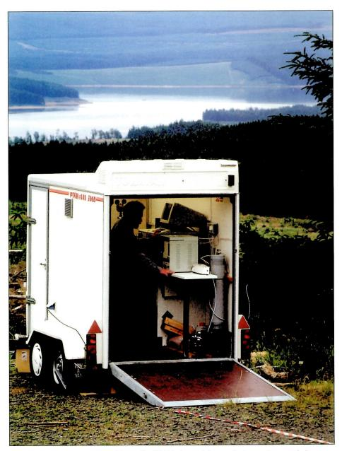
*Plate 27.* Mobile laboratory used by staff at ITE Merlewood for monitoring methane and nitrous oxide fluxes
