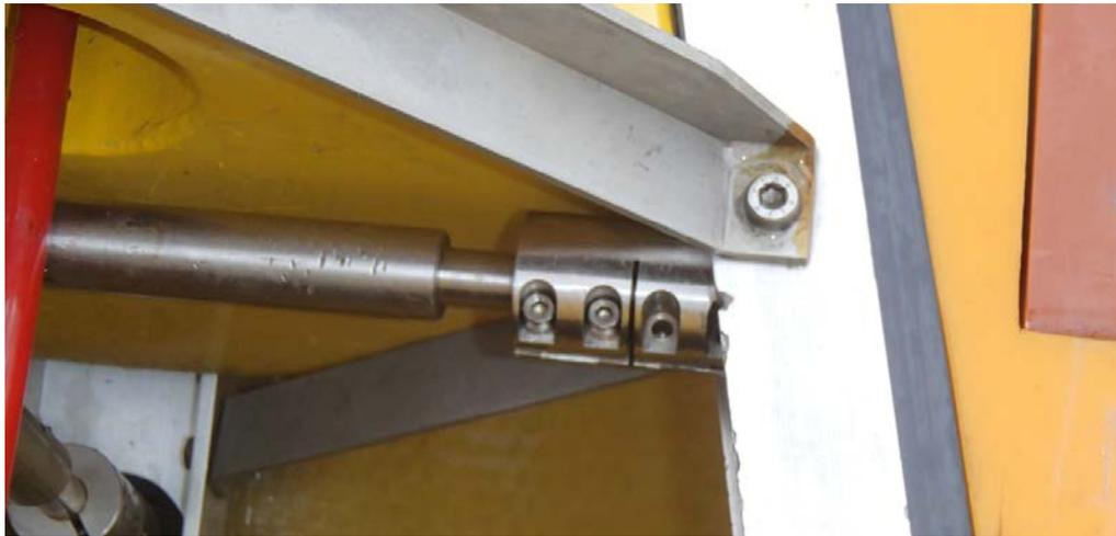
Figure 19.15. Port side coupling outer portion was slipping during M463 (note the bolts removed in this picture were in place during the deployment)
