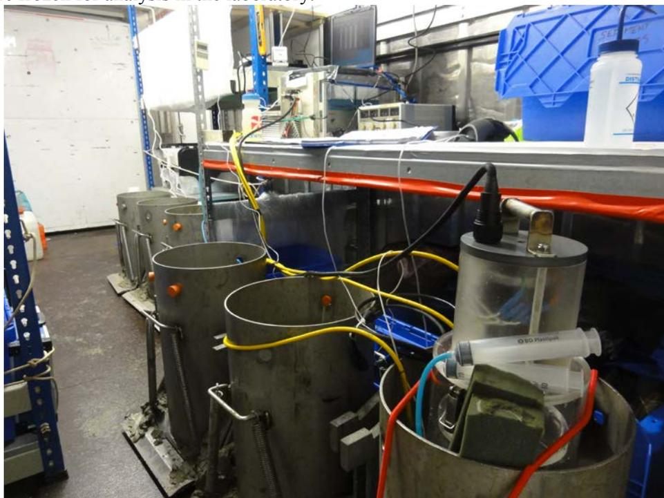
**Figure 1:** Core Mini Flume in place during the resuspension experiments
