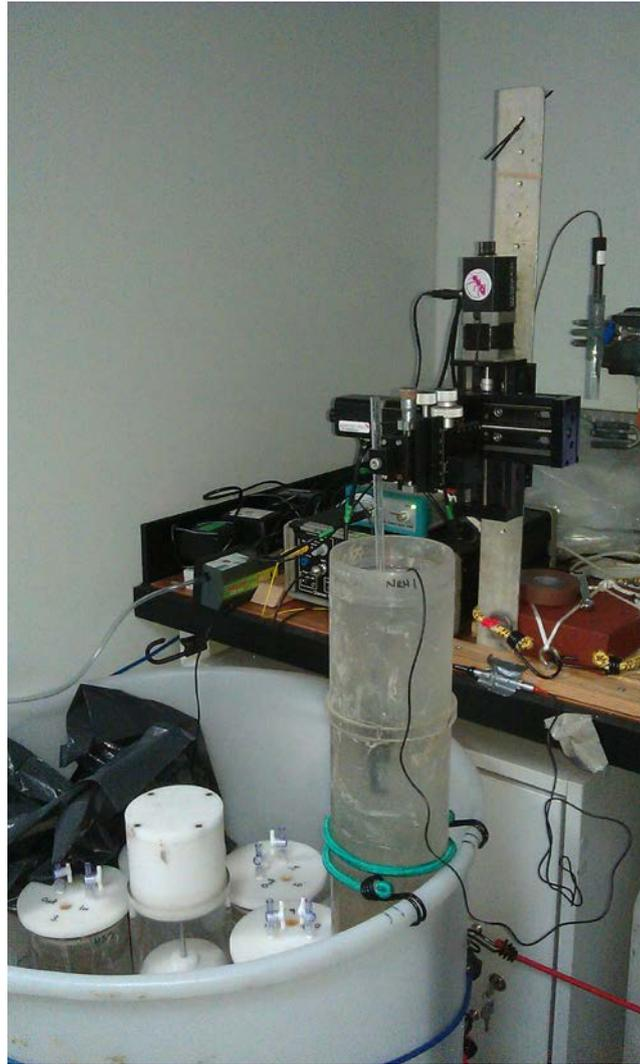
Figure 17.1. Showing the sediment incubation and profiling setup in the CT room.
