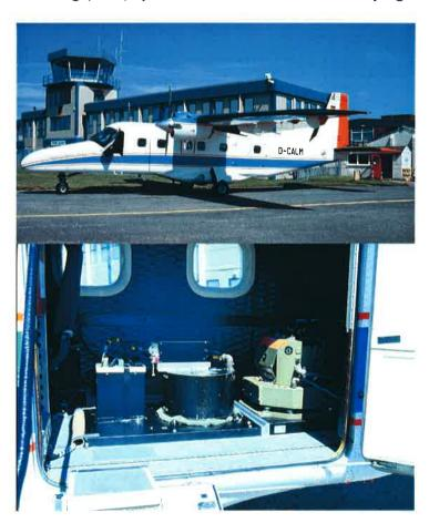
Figure 1: The NERC ARSF Dornier 228 Airborne Remote Sensing Platform, with CASI, AZ-16 ATM and RC-10 instruments.
