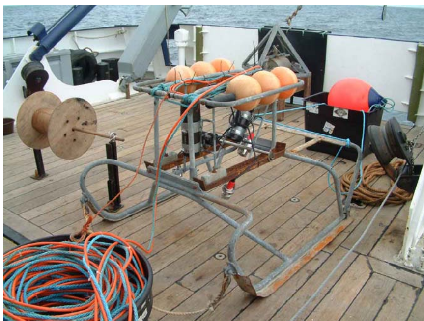
FIGURE 1 Camera sledge with Photosea still camera system (black housings), and Rovtech video camera and lights (red plug retainers). The umbilical cable is coiled in the tub on the left and the tail rope buoy is to the right.
