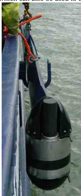
Reson 8101 transducer mounted on the pole (left). Multibeam data acquisition and processing set-up during geophysical survey (top). Photos Dave Smith, BGS.
