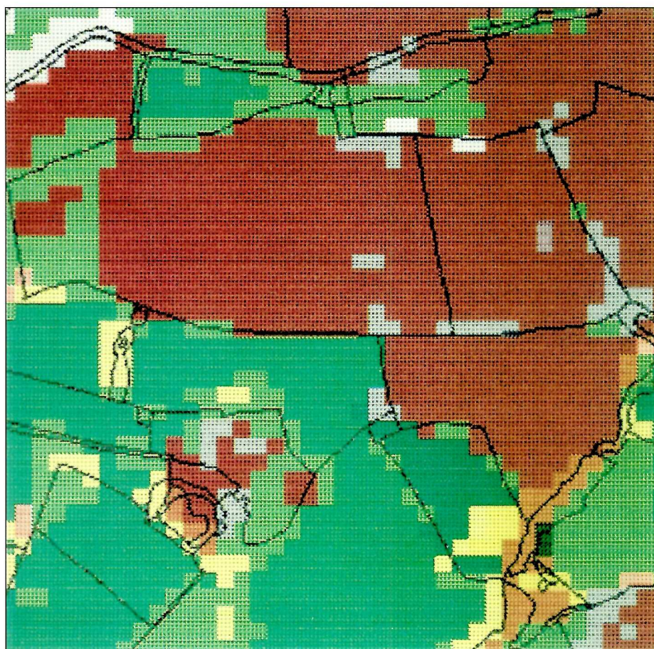
Figure 65. Use of digital maps of field survey to assess the accuracy of land cover mapped from remote sensing. The Figure corresponds to 1 km square near Newmarket, Suffolk. The remotely sensed land cover map appears as the coloured gridded underlay (brown=arable land, light green=grassland, dark green=coniferous woodland, buff= deciduous woodland, yellow=heathland, grey=buildings). The linear overlay results from digitising landscape features mapped in the field. Accuracy assessment involves comparing the contents of the digitised land parcels (held separately in a data base) with the remotely sensed map, and drawing up a matrix to compute the degree of correspondence between the two
