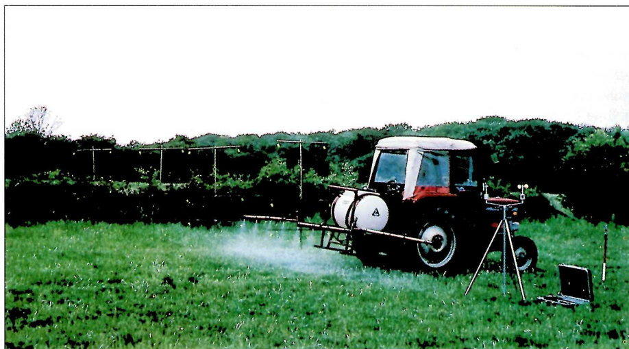
Plate 12. Tractor spraying 6 m upwind of a hedge with an array of receptors to collect drift
