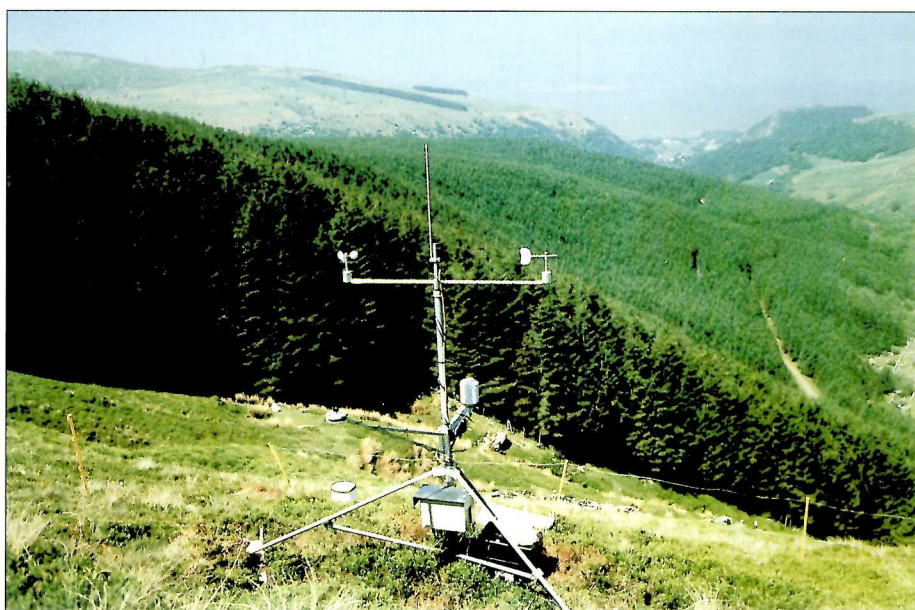
Plate 9. An automatic weather station outside a forest plantation in north Wales
