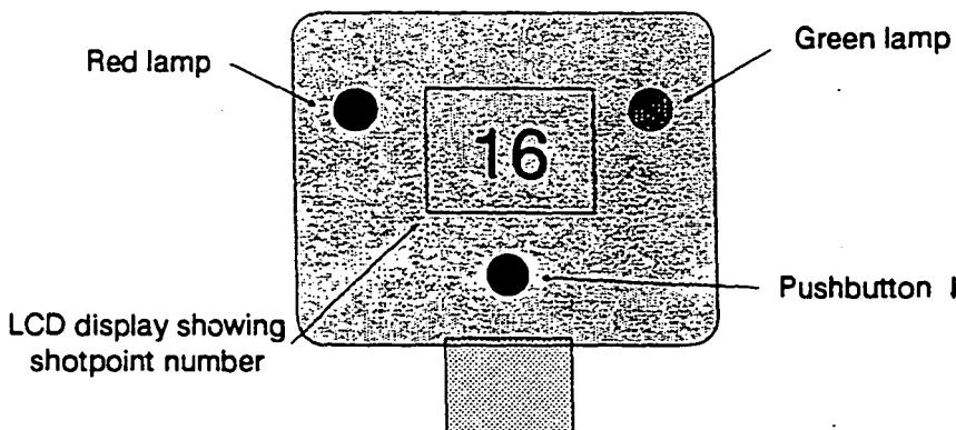
Fig 2-5. The Remote Control Unit (Top view)
