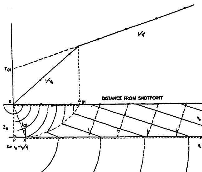
Fig 4-4. Spherical and diffracted wave fronts with ray paths.
