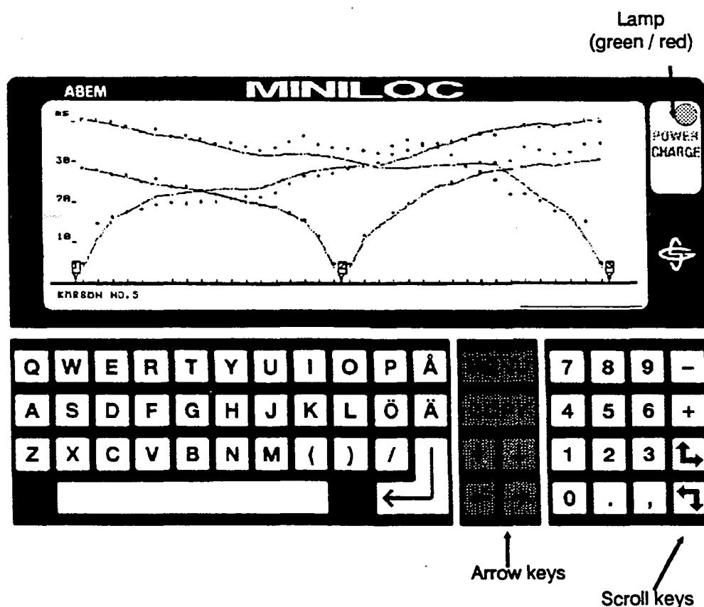
Fig 3-1. The MINILOC keyboard with the graphic LCD display.
