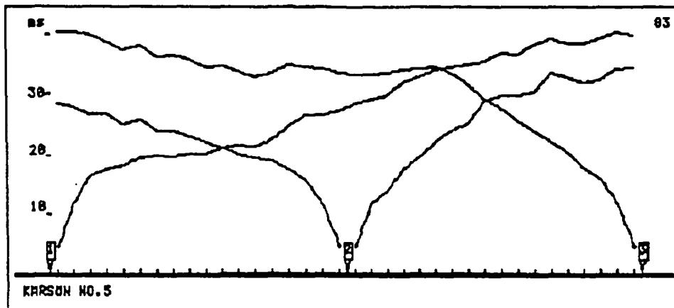
The quality of the data appears immediately in this display. the curves should be rather smooth, without any "dropouts". Whenever you observe X-T curves of dubious quality, go back to the edit menu (MENU 82) and check and adjust the data point.
