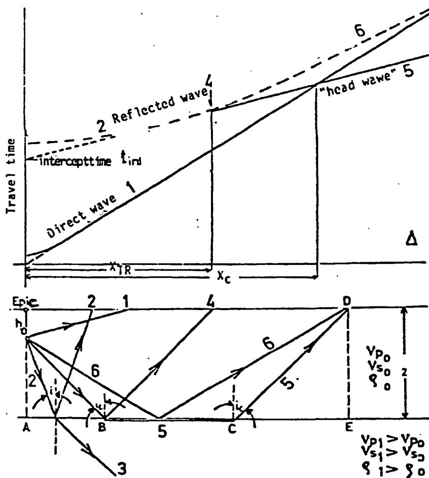
Fig 4-5. Seismic wave paths and traveltimes in a two-layer case.
