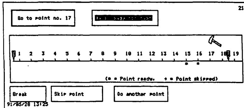
From this point the MINILOC is controlled from the Remote Control Unit (RCU), which will display the number 1. Now you can go to shotpoint 1 and start shooting.
