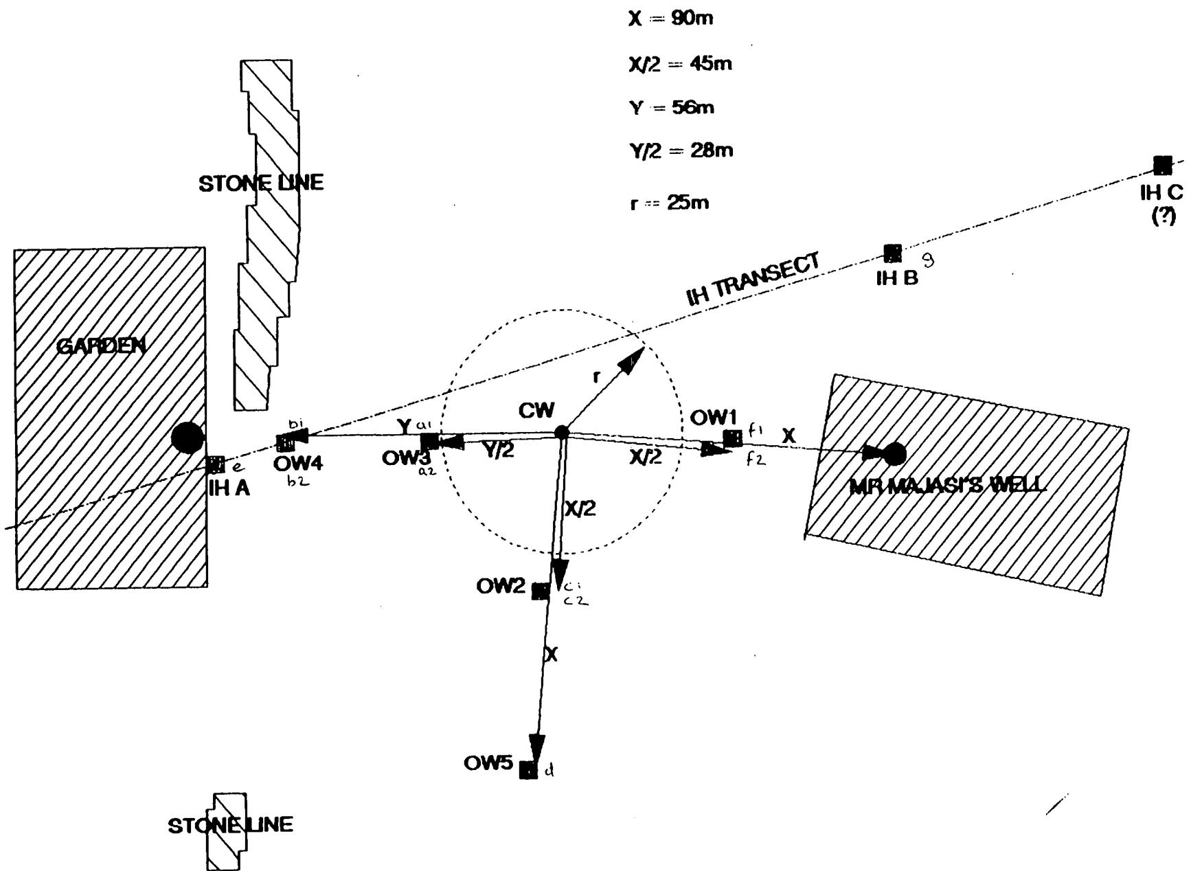
Fig Observation boreholes drilled adjacent to the Tamwa Collector Well (after Price, 1992).
