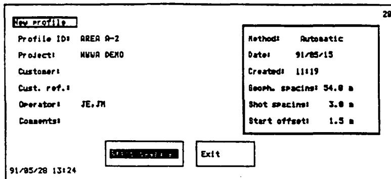
When satisfied with the settings, go back to the main menu and choose AUTOMATIC to perform a standard survey with the standard cable. This brings up the above menu, in which necessary information about the survey is specified. The most important position is the **Profile ID** which is used for identification later on. When finished, choose the **START MEASURE** option, which will bring up the data collection menu with the hammer.
