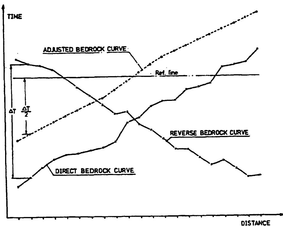
*Fig 4-7. Average refractor velocity determination. The adjusted bedrock curve is the result of the MMT calculation.*
