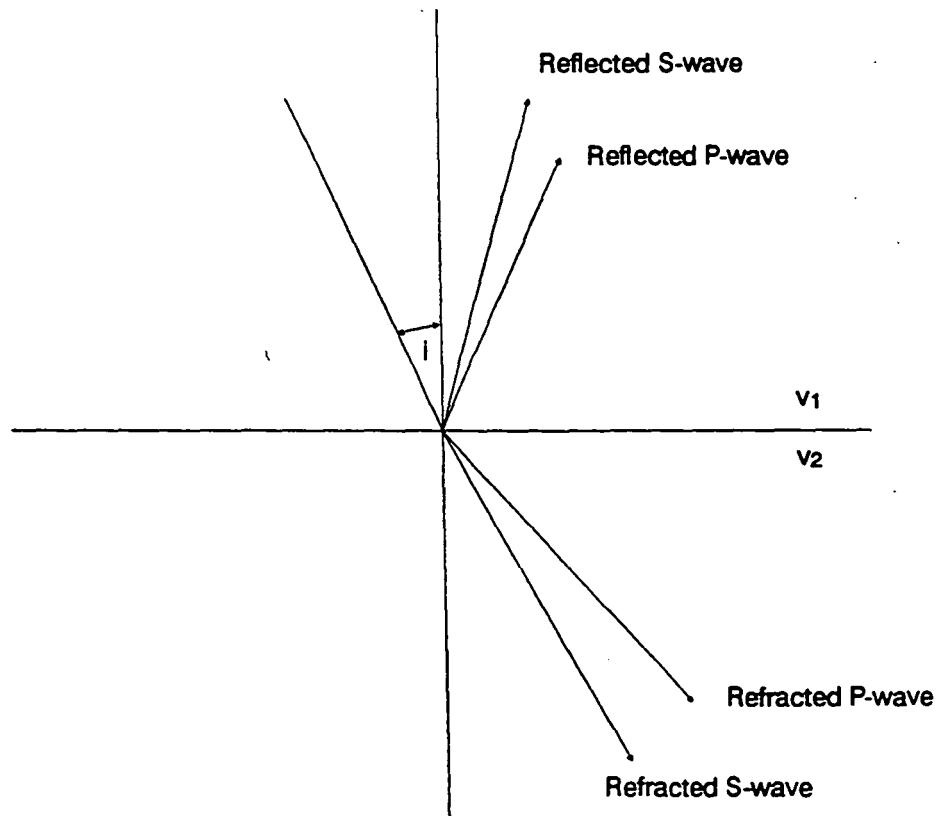
Fig 4-3. Reflection and refraction at a seismic boundary.
