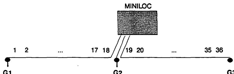
Fig 3-1. MINILOC layout with geophones G1, G2 and G3 and shotpoints 1 to 36.
