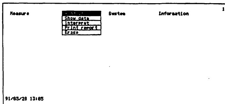
When you have finished the profile it is time for processing. The first step is to go to *PROFILE* and choose *SHOW DATA* to check the data quality.
