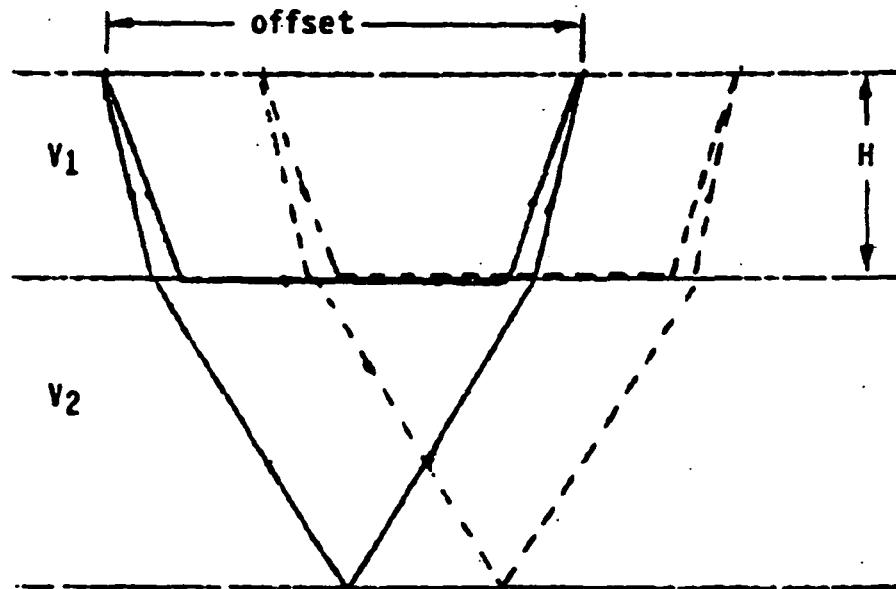
Fig 4-11. Raypaths for two common offset shots showing reflected and refracted waves.
