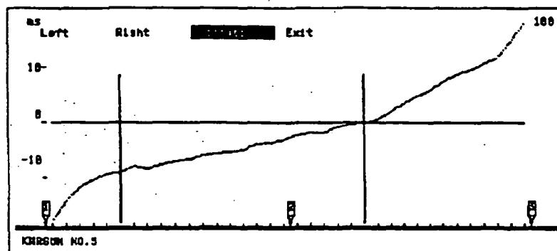
as the right border. When finished select COMPUTE. This implies the optimization program to use the velocities from the MMT calculation instead of a constant velocity. A low-velocity zone in the lower refractor is indicated on the model display by a hatched line.
