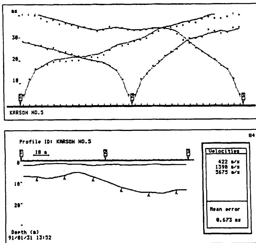
Data fitting (upper diagram) and corresponding model (lower diagram). The mean error is defined as the total deviation between the measured data and the response, divided by the number of data points (108). A value less than 1msec means that the fitting is very good.
