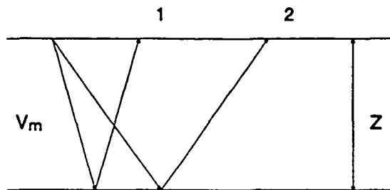
*Fig 4-6. Reflection at horizontal boundary.*
