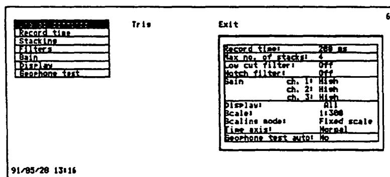
The gain is always controlled automatically in the program. However, when using the manual monitoring in the TRIG option, the gain setting is of importance. It can be set to HIGH or LOW. To the right of the display, all settings are displayed.
