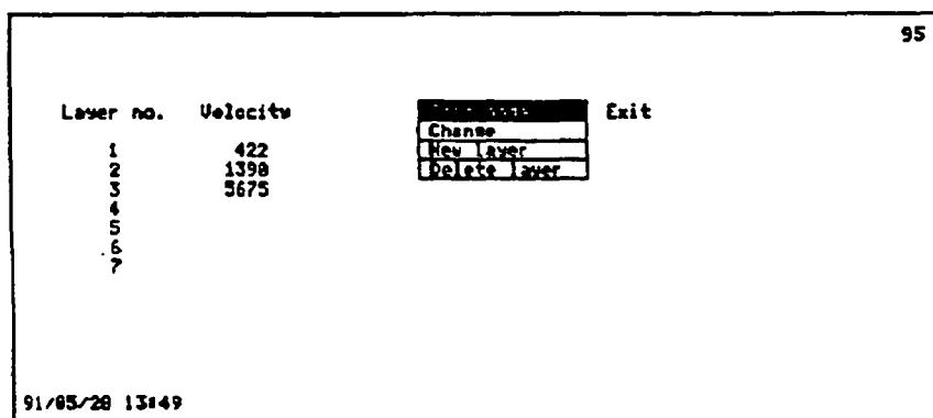
*PROFILE* and *INTERPRET*, and the interpretation menu will appear. Choose the option *START MODEL*, and the program will calculate appropriate velocities for a number of layers (up to 7 layers). When finished (after a few seconds) the program will display "DONE", and you can
