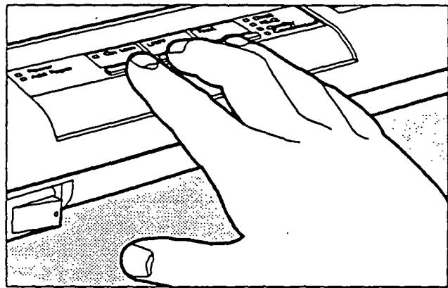
3. Allow the batteries to charge until the Font indicator stops flashing and the Power indicator comes on. (Recharging can take 10 to 14 hours.)
