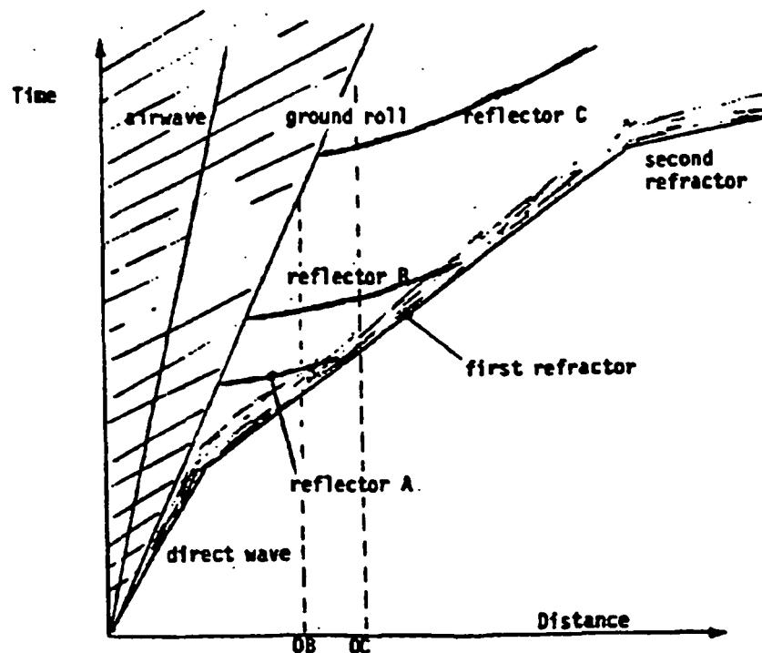
*Fig 4-10. Time-distance graph showing the positions of important events. The "window" between OB and OC is suitable for Common Offset measurements.*
