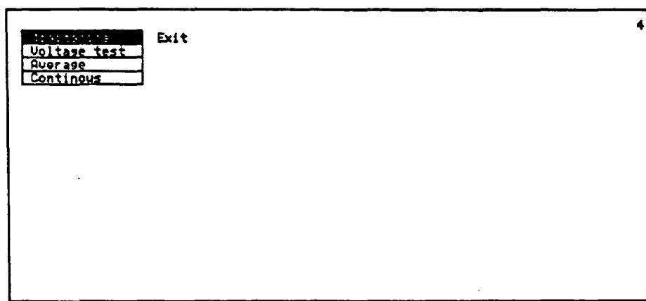
Fig 2-4. The SELF TEST menu with the three choices for voltage monitoring. Select VOLTAGE TEST to display the battery voltage.
