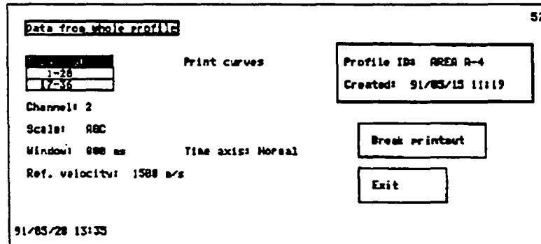
Observe, that *REF VELOCITY* is used in reflection seismics, and of no importance in refraction seismics.
