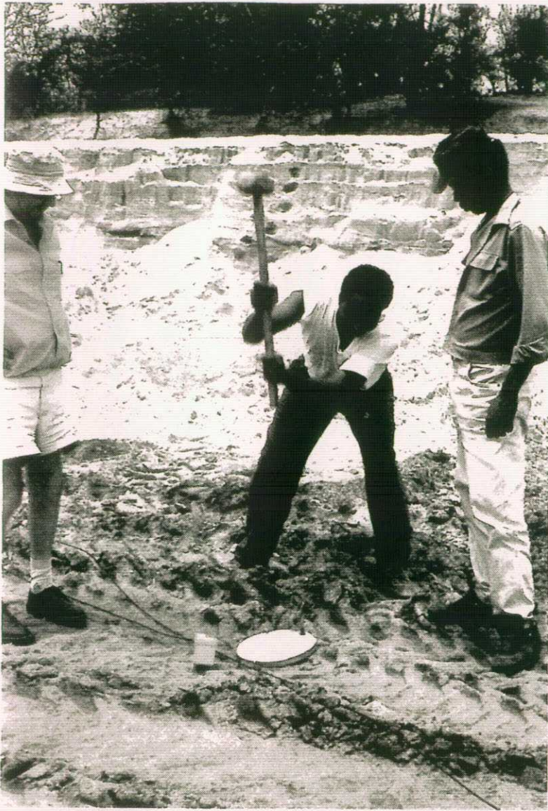
Figure 6 Production of a seismic signal, by hammering an aluminium plate adjacent to a triggering device.
