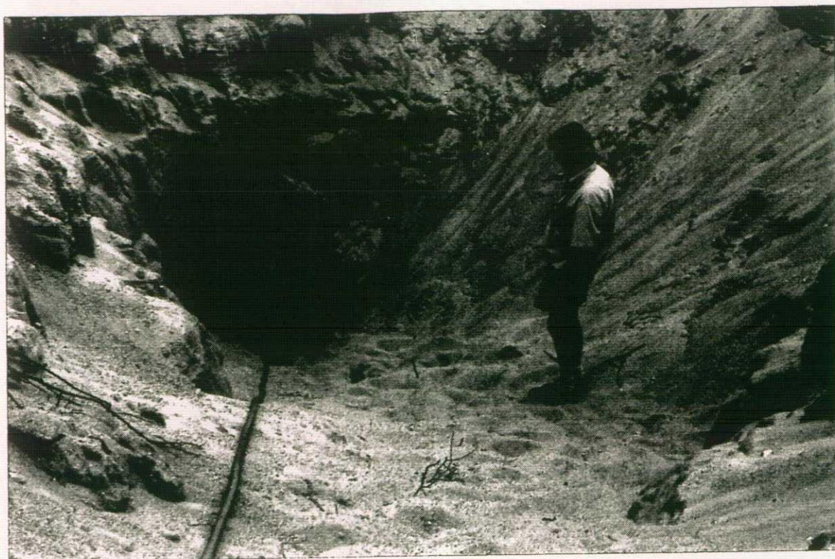
Figure 9 Jetting monitoring well, for aquifer flow determination using salt dissolution, into the basal saturated zone at the bottom of a cattle watering hole at Masunga site A
