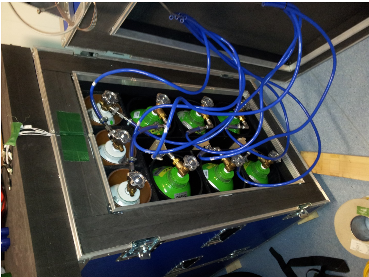
Figure 25: Photograph of the cylinder Blue Box, showing three 10L working tank cylinders (top row) and six 20L cylinders used for calibrating the system.
