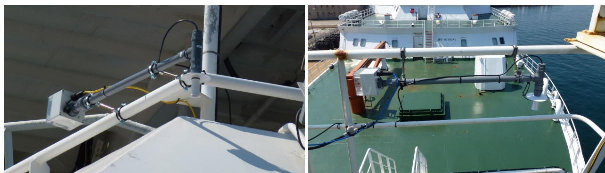
Figure 22: Photographs of the aspirated air inlets on the monkey island (left) and the foremast (right).
