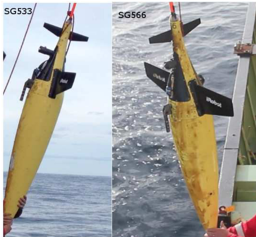
Figure 6: (Left) 533 being recovered with the rope wrapped around half the rudder and the antenna. (Right) 566 being recovered with the rope wrapped around half the rudder.
