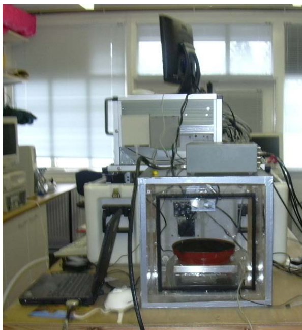
Figure 1.54. Photograph of the cuvette setup used to quantify \text{HNO}_3 emission from slurry under semi-controlled conditions.
