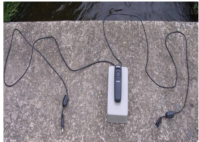
Figure 1. Camera synchronization- relay switch and cords
