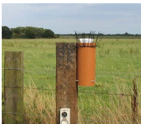
Figure 4 Bulk Precipitation collector at Heigham Holmes with cable tie bird scarer ring.
