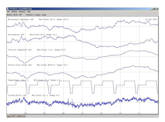
system. GDASView is a Javabased, Microsoft Windows utility for retrieving, recording and plotting data from a remote observatory GDAS recorder; while the SDAS acquisition software provides an HTML interface, for monitoring and
