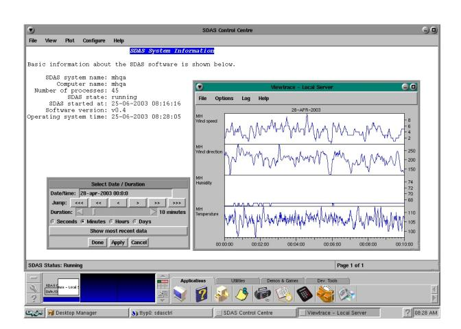
acquisition software can be controlled and data plotted locally using a graphical user interface running under QNX Photon. BGS has also developed software, including a set of Java classes, for remotely maintaining an observatory
