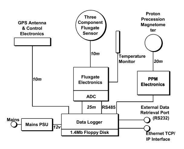
available for dissemination through either a network port, RS232 serial port or floppy disk. The processor and the sensors are powered by a single mains-voltage supply with a 24 hour battery reserve. The architecture of the operating system and the design of the acquisition software provide a versatility that allows new sensors to be readily incorporated such that
