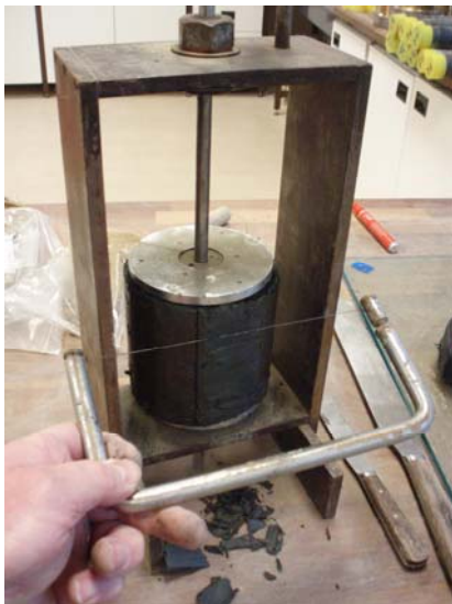
Figure 11 Preparation of undisturbed specimen using wire saw and guide (100mm).
