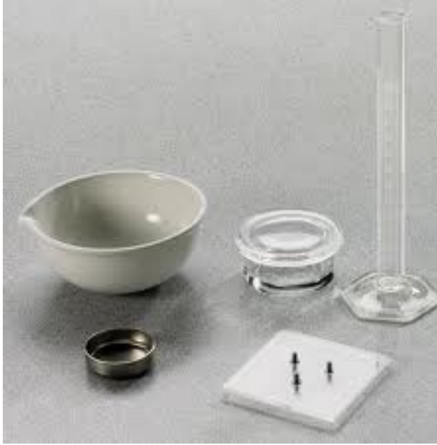
Figure 4 'ASTM' 'prong plate' shrinkage limit test apparatus (BS1377:1990, Part 2, Test 6.4)
