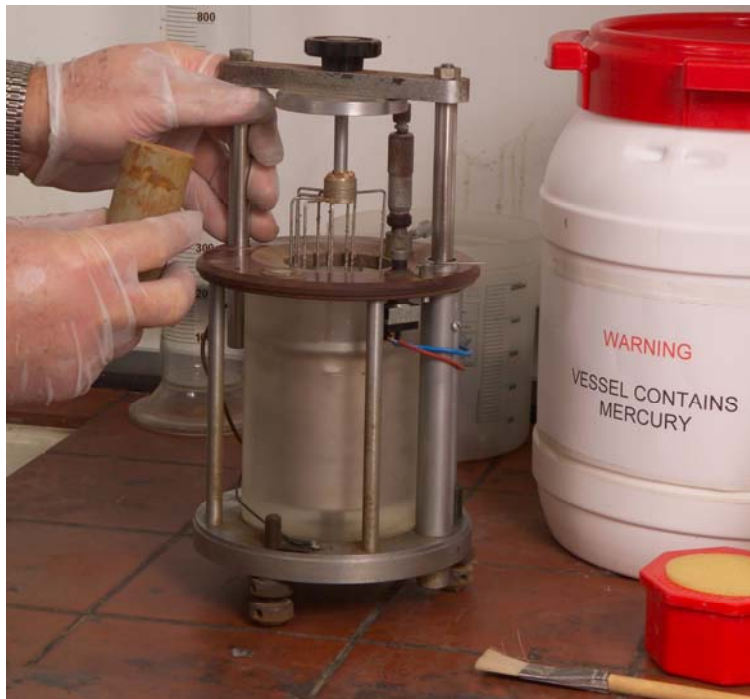
Figure 3 ‘TRL’ shrinkage limit test apparatus ( BS1377; 1990; Part 2, Test 6.3 )
