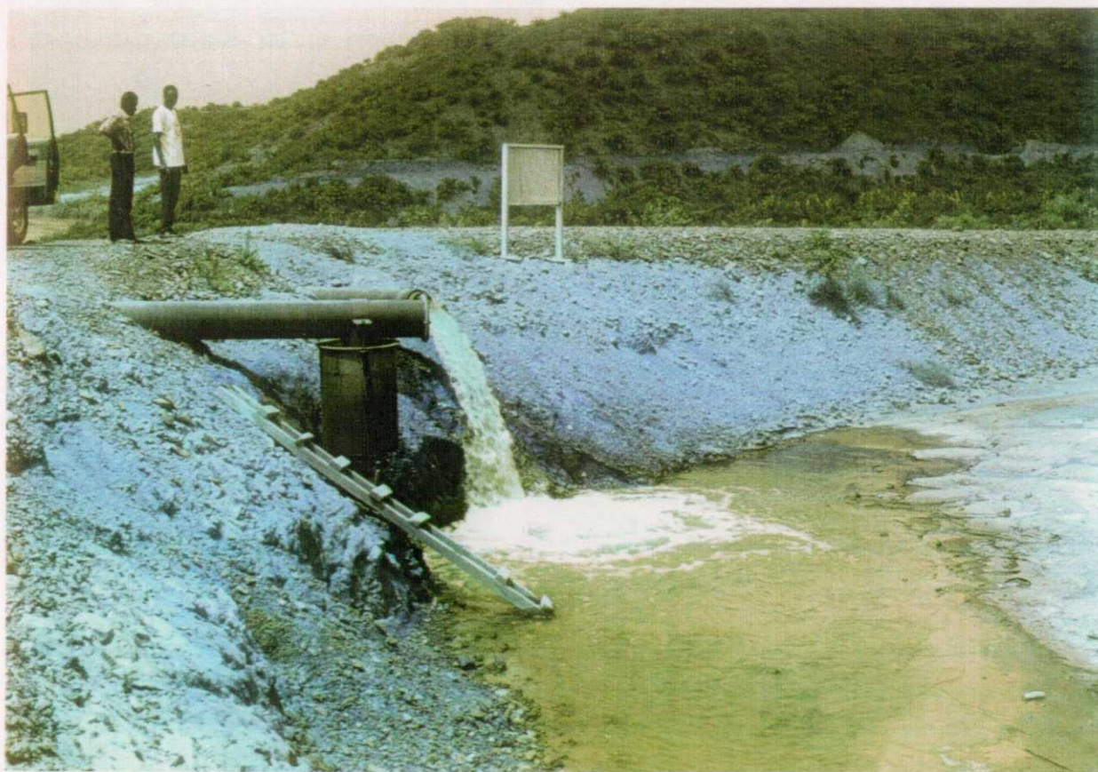
Plate 2.2. Tailings effluent from a nearby tailings dam being pumped directly into the Kwabrafo stream. Tailings effluent is now recycled rather than discharged.
