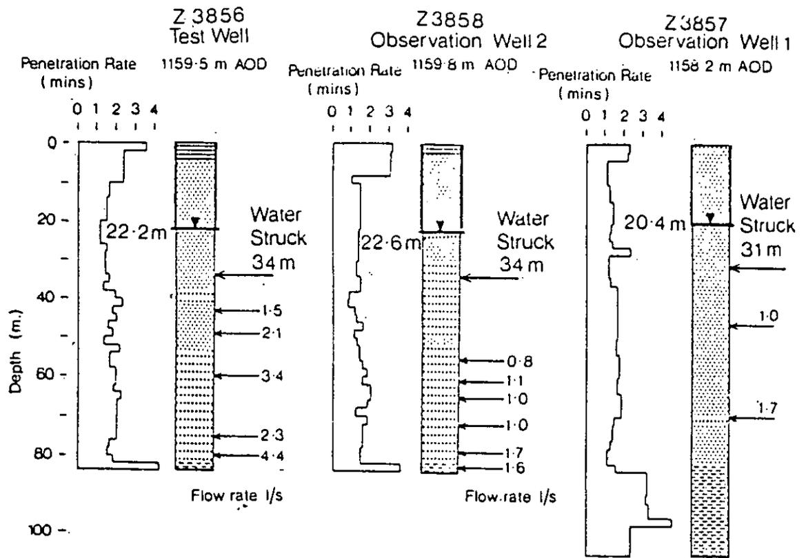
TEST SITE TS SYC LITHOLOGY AND DRILLING DETAILS
