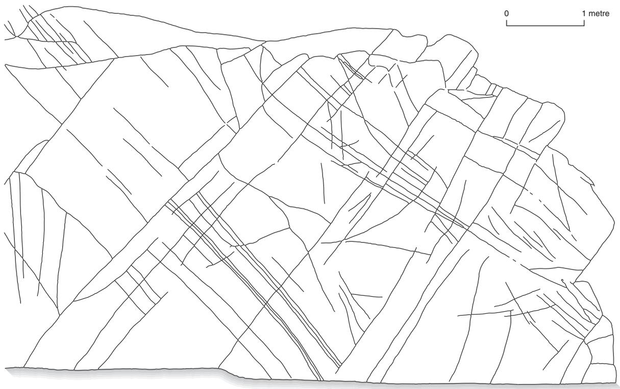
**Figure 9** Example trace map of a **discontinuity-network** displayed on a near-vertical exposure surface in a felsite intrusion, Gosforth, Cumbria. The face is inclined  $84^\circ$  south-south-east, and two discontinuity sets are evident: one has 10 cm- to m-range spacing, with an apparent dip to the west (left); in the other set, discontinuities with cm- to 10 cm-range spacing and a gentle/moderate apparent dip to the east form clusters with m-range spacing.
