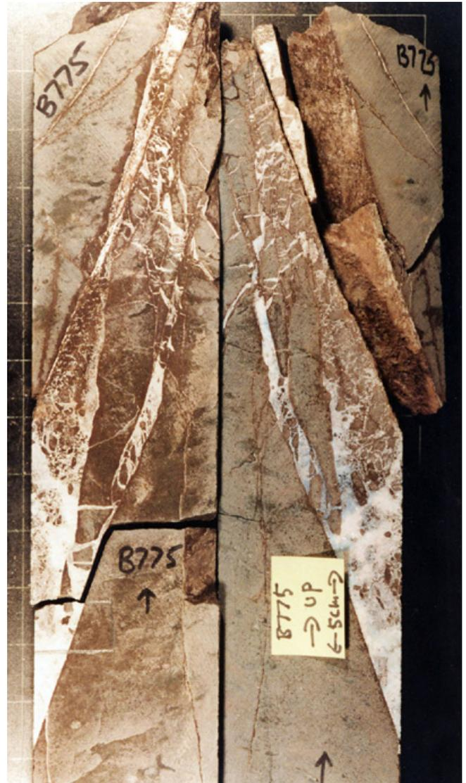
**Figure 15** Example description of filled discontinuities in a longitudinally sliced section of borehole core, 9 cm wide and 30 cm long, in greyish green volcanoclastic rock; acid etching and staining of the right-hand side has been used to help identify carbonate minerals in fractures.
