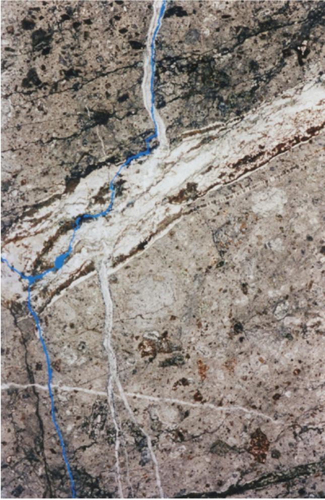
**Figure 18** Example description of filled discontinuities in a 2 x 3 cm area of blue-dye resin impregnated thin section prepared from altered volcaniclastic rock.
