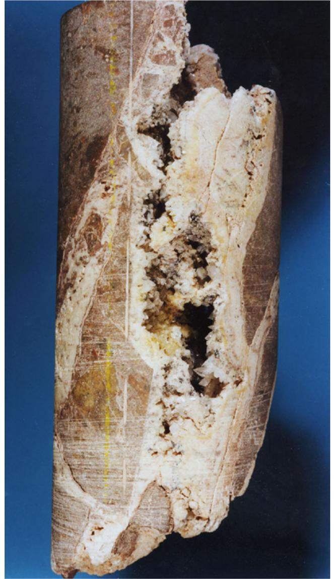
**Figure 17** Example description of a partly filled discontinuity in borehole core.
