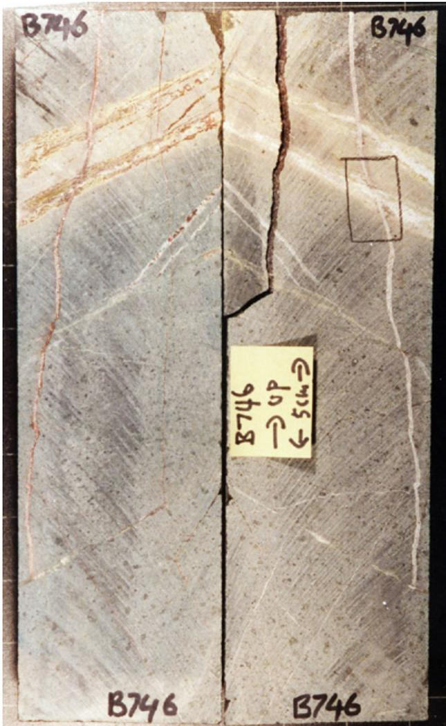
**Figure 14** Example description of filled discontinuities in a longitudinally sliced section of borehole core, 9 cm wide and 30 cm long in greyish green volcanoclastic rock. Acid etching and staining of the left-hand surface have been used to identify the carbonate minerals in fracture fillings.
