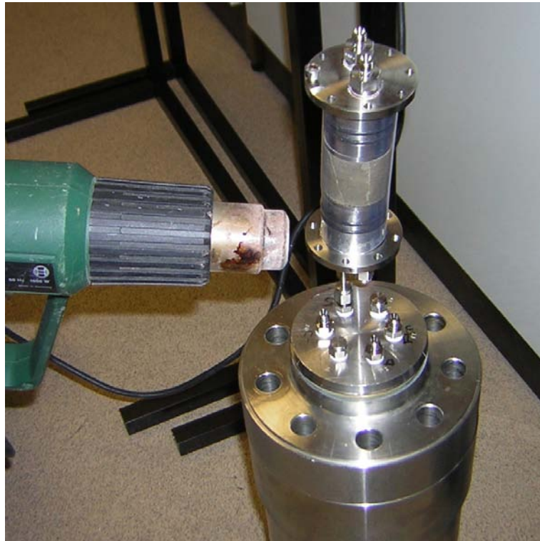
Figure 4 Use of heat gun to shrink tubing around cut core. (Biotic experiment)
