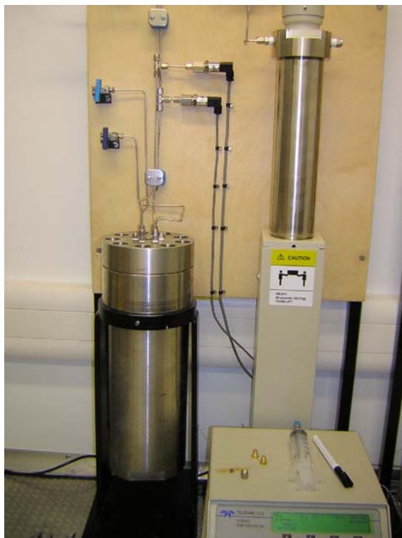
Figure 8 Fully completed apparatus showing the attached pump assembly (Biotic experiment).
