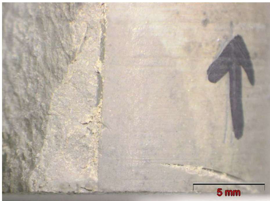
Plate 9 Binocular microscope photomicrograph showing annulus channel in the outer wall of the core plug where a fragment of the opposing fracture wall has fallen away. Post-experimental material. (Biotic experiment).
