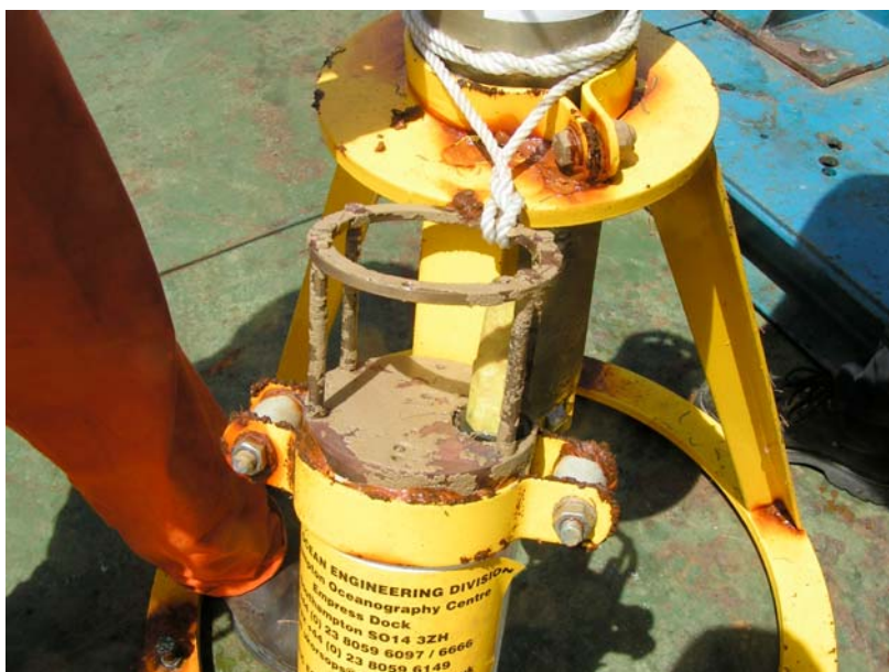
Photograph C.10: Fouling on EBH4 tripod and BPR
