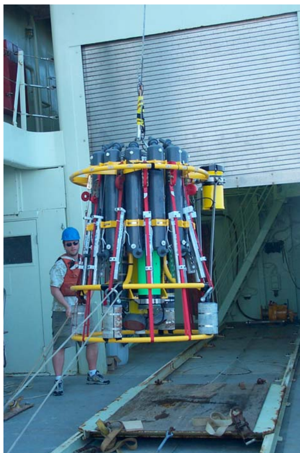
Photograph C.22: Microcats attached to CTD frame for calibration on KN182-2. Attached using ratchet straps.
