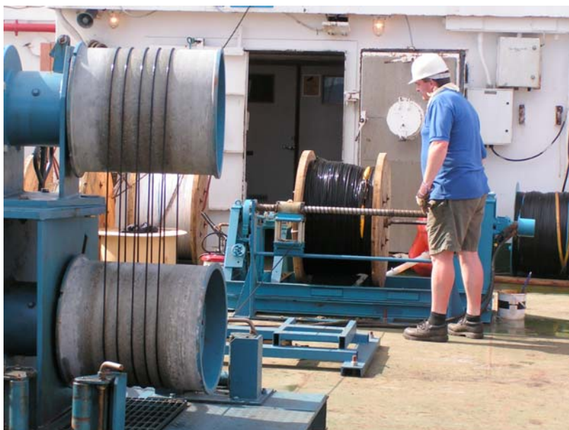
Photograph C.4: Double Barrel Capstan (DBC) with extended reeler holding a wooden storage drum
