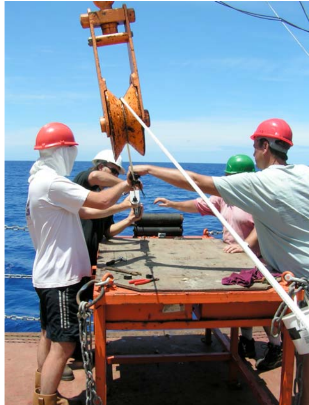
Photograph C.6: Mooring Table – Attaching an SBE37 Microcat
