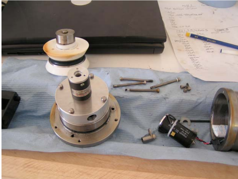
Photograph C.17: MAR4 MMP drive motor internals. – The gearbox was sheared off the motor and all end cap screws were badly bent.
