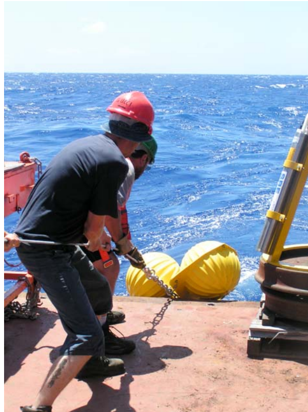
Photograph C.12: Hand deployment of a glass buoyancy package, on EBH2, with the rails down
