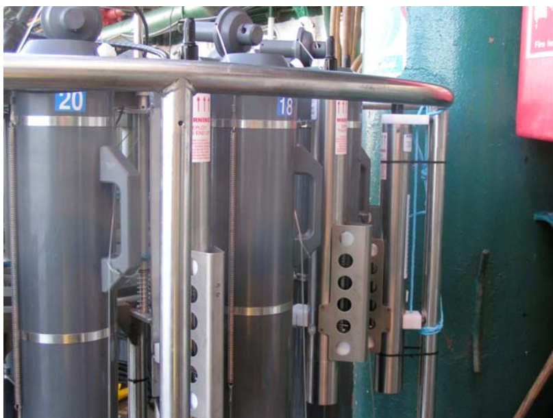
Photograph C.20: Microcats attached to CTD frame for calibration on CD170. Fixed using bespoke brackets.
