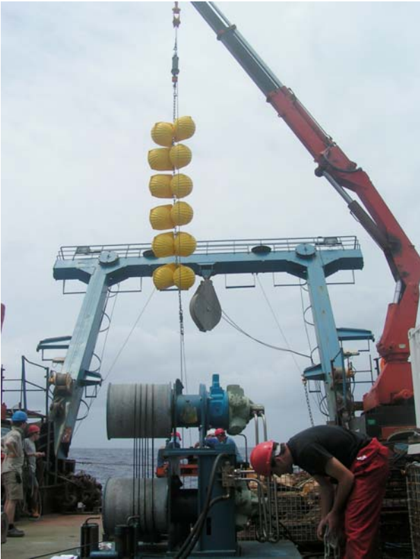
Photograph C.5: Raft of glass floats lifted with ship's crane
