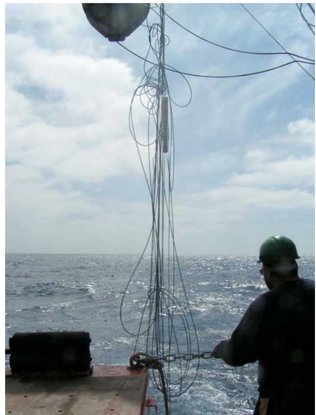
Photograph C.14: Wire wuzzle during EB3 recovery
