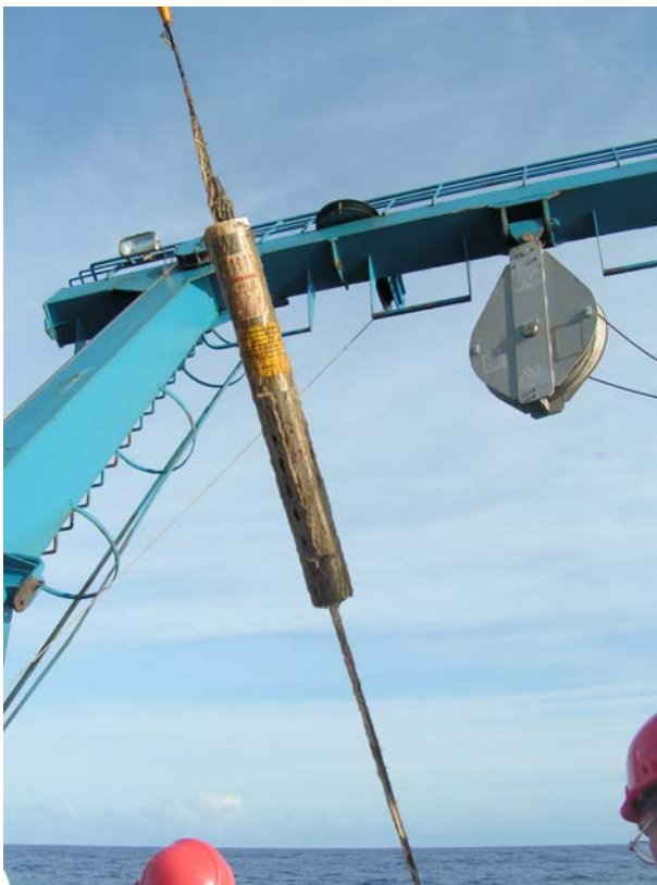
Photograph C.18: Heavy fouling on Microcat at 50m depth on MAR1 mooring
