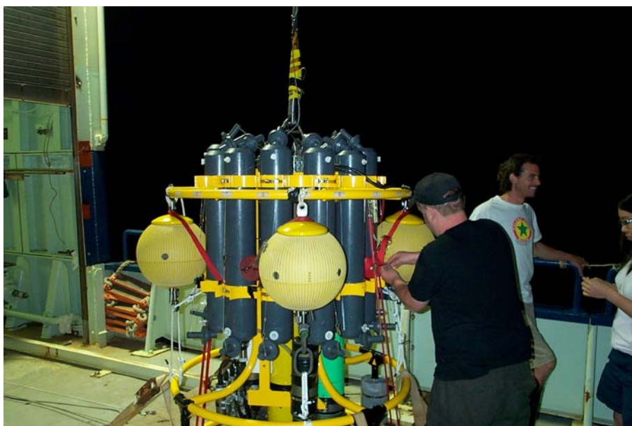
Photograph C.23: S4 current meters attached to CTD frame for calibration on KN182-2.
