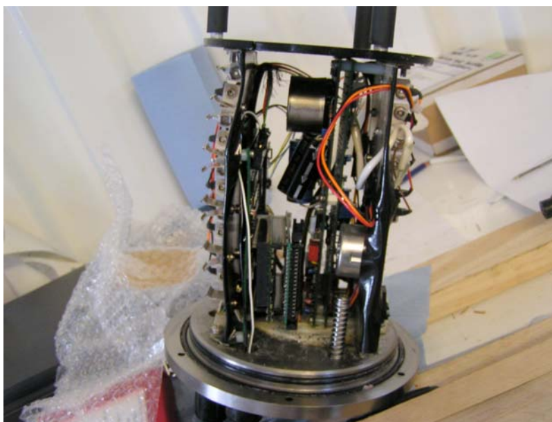
Photograph C.16: MAR4 MMP internal electronics chassis badly distorted, with electronic components broken off boards
