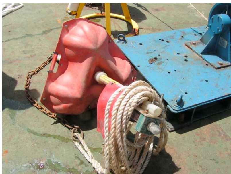
Photograph C.9: Fouling on EBH4 Billings float and recovery line
