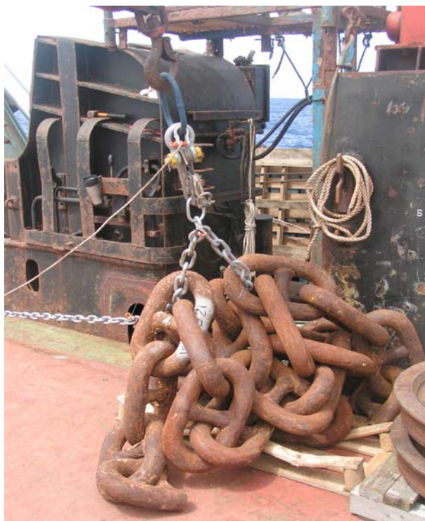
Photograph C.8: Seacatch release hook lifting a 1.25 tonne anchor clump
