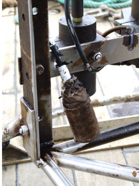
Figure 4 - UoL metal ion probe head and chaffing on CEFAS instrument
