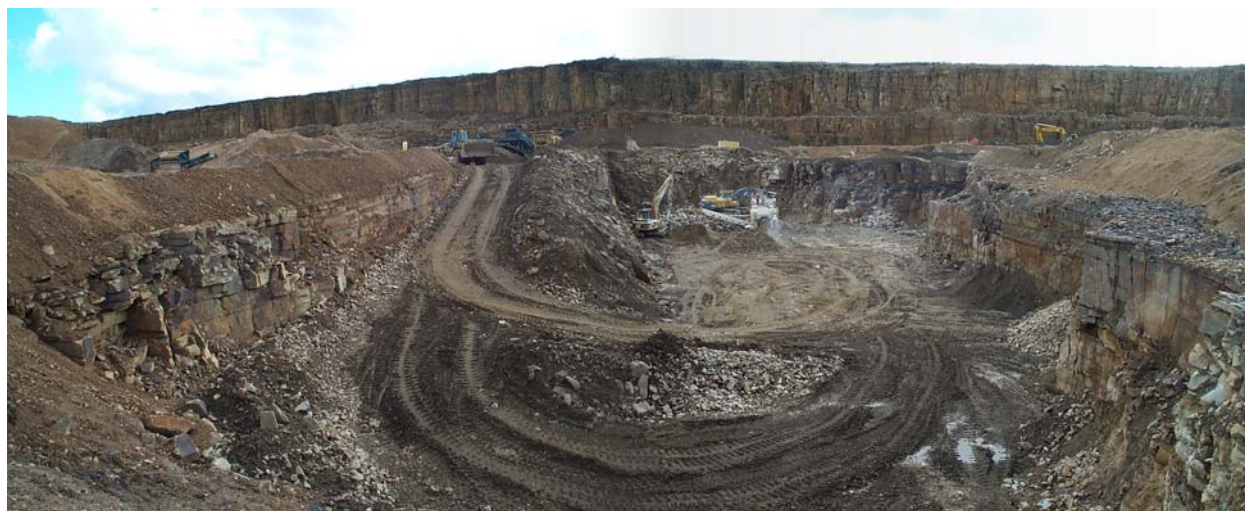
Figure 5. Hanson Aggregates: Brinscall Quarry, Chorley, Lancashire; Carboniferous, Fletcher Bank Grit is worked for crushed rock aggregates. Photo courtesy of Hanson Aggregates.
