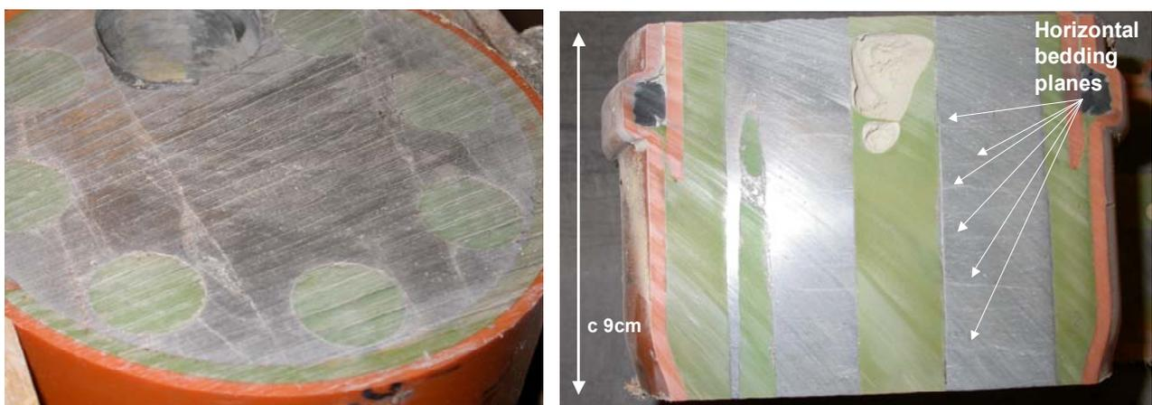
**Figure 3 – Vertical (1) and horizontal (2) fractures running through the supplied core.**
