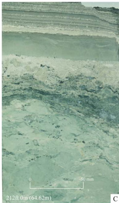
Plate 3. Wiscombe Park No. 1 Borehole: selected Dunscombe Mudstone Formation lithologies.
