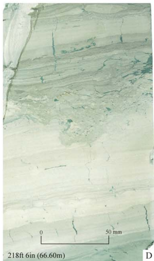
Plate 3. Wiscombe Park No. 1 Borehole: selected Dunscombe Mudstone Formation lithologies.
