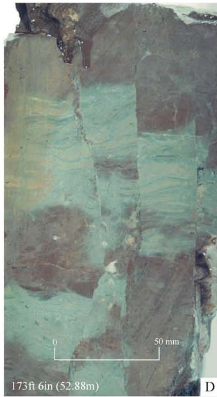
Plate 4. Wiscombe Park No. 1 Borehole: selected Dunscombe Mudstone Formation lithologies.
