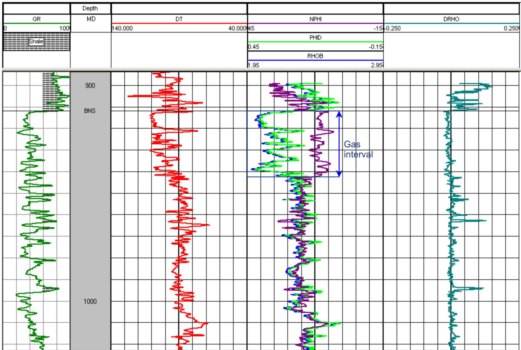
Figure 4: Gas effect at the top of the BNS in well 52/5-3.
