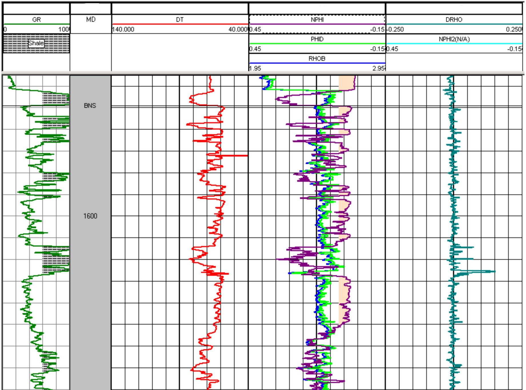
Figure 5: Salt cementation in the BNS (shaded orange on the NPHI log) in well 49/16-7Z
