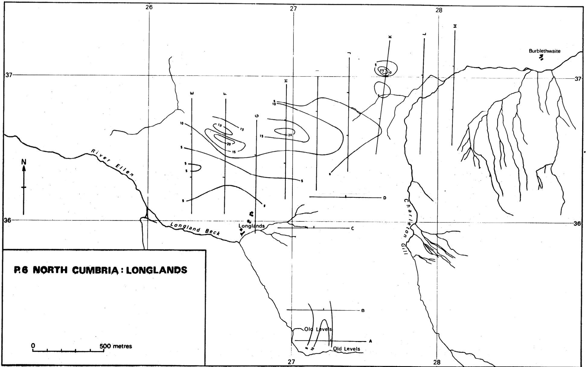
Fig. 22. Chargeabilities in milliseconds at  $n = 4$ , Longlands
