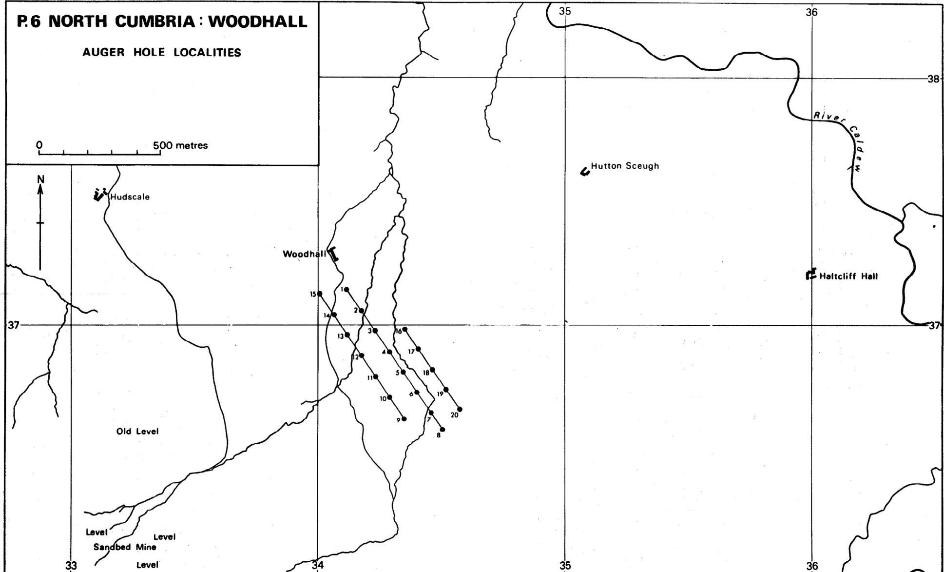
Fig. 7 Location of auger holes, Woodhall
