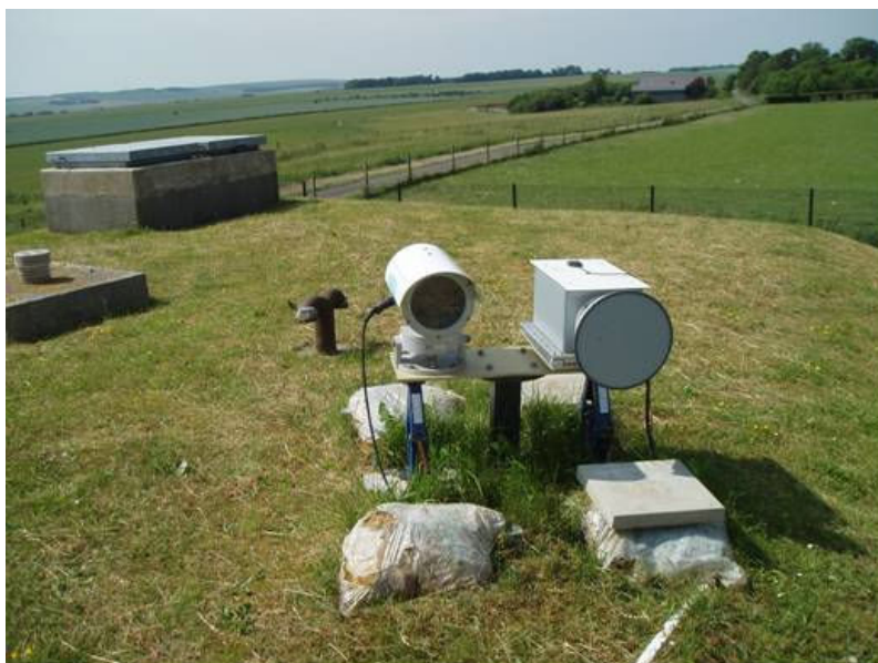
Figure 5-1 The Kipp and Zonen LAS 150 (left) and the CEH-RAL MWS (right) – the LAS-MWS two-wavelength scintillometer system. Shown is the receiver site at Stancombe Reservoir.
