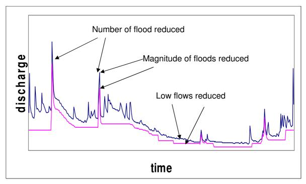
Figure 1 Indicators of Hydrological Alteration (after Richter et al. 1996)
