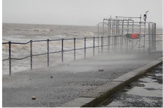
Figure AIII.10: Example of debris overtopping the wall during WireWall deployments. Debris found on arrival at site morning of the 8 th November 2018 (left). Brick debris overtopping south of the rig during on the 22 nd January 2019 (right).
