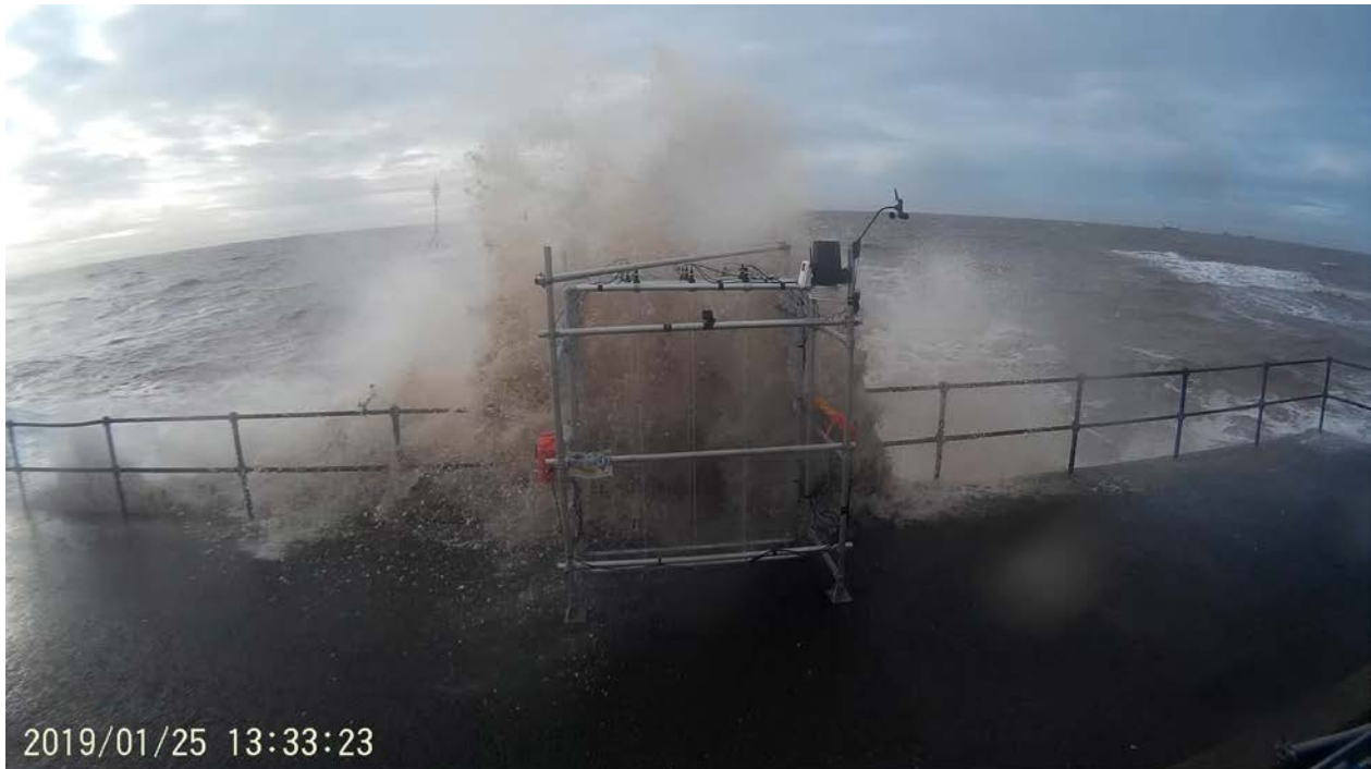
Figure 4.23: Still image of one of the very largest plumes observed during the deployment on Friday 25 th January 2019. It can be seen that the seawards part of the plume is taller than the rig. However, the upper part of the flume is made up of quite fine spray compared to the much denser spray/solid water lower down. In addition, the height of the plume reduces as it travels through the rig.
