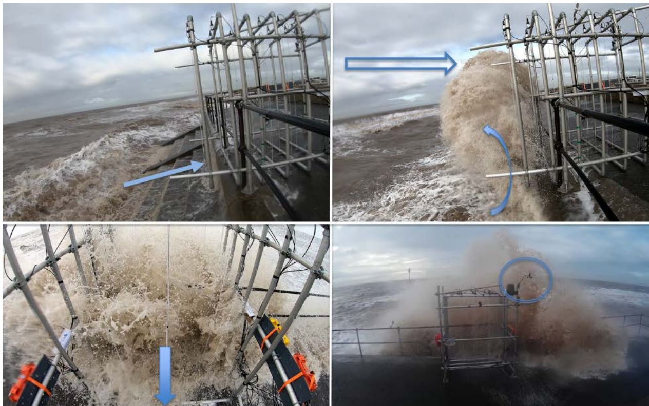
Figure 4.21: Example photo sequence to explain the site-specific processes during a typical windy spring tide that potentially require an alert to be issued for pedestrian safety, but are not represented within generic hazard warning tools. The position of the weather station is also shown (bottom right).
