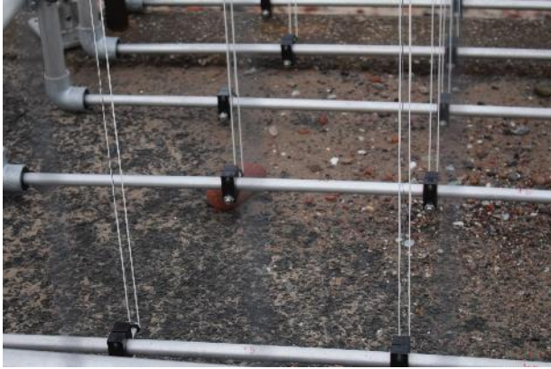
Figure AIII.10: Example of debris overtopping the wall during WireWall deployments. Debris found on arrival at site morning of the 8 th November 2018 (left). Brick debris overtopping south of the rig during on the 22 nd January 2019 (right).
