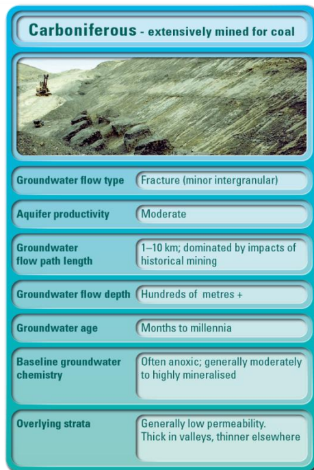
Figure 38 Overview of the hydrogeology of Carboniferous aquifers in Scotland that have been extensively mined for coal: (top) schematic cross-section; (bottom) summary of aquifer characteristics. From Ó Dochartaigh et al. (2015).
