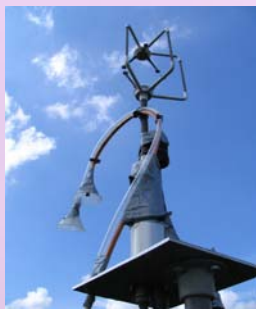
Fig.1 Arrangement of the inlet lines close to the ultrasonic anemometer (PTFE for the gases: N 2 O, CO 2 , H 2 O, VOCs, copper tube for aerosols).
