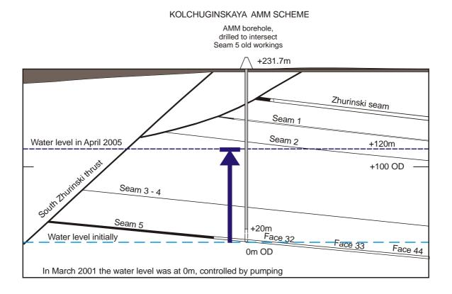
Figure 17. Sketch cross-section of the AMM scheme at the Kolchuginskaya Mine. Redrawn from an original kindly supplied by Gorsh.
