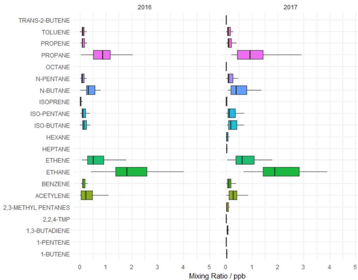
**Figure 86. Box and whisker plot of NMHCs measured at KM in 2016 and 2017.**
