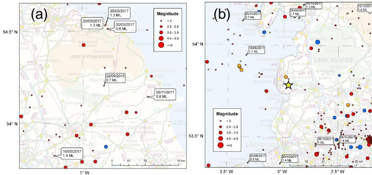
**Figure 27. Earthquake activity in 100 km squares centred on Kirby Misperton (a) and Preston New Road (b). Earthquakes in the time period from 1/4/2017 to 31/3/2018 are marked by yellow circles. Circles are scaled by magnitude. © Crown Copyright and/or database right, 2018. Licence number 100021290 EUL**
