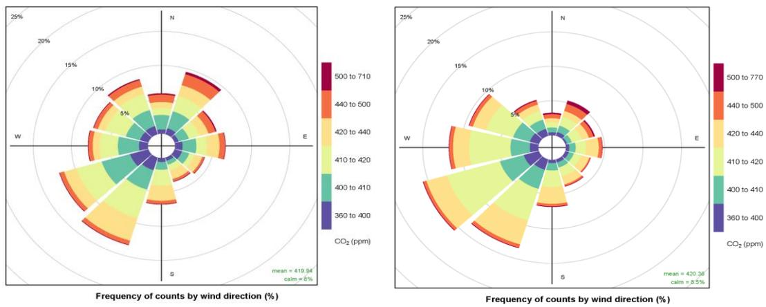
**Figure 53.** Concentration (as per colour scale) wind rose for carbon dioxide as measured at KM in the 2016–17 baseline period (left) and 2017–18 period (right). Radial extent contours define 2% frequency intervals. © University of Manchester, 2018
