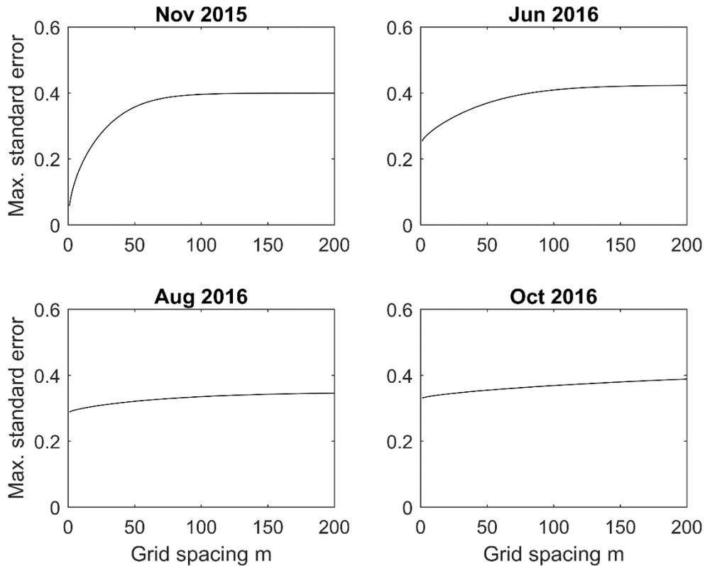
**Figure 117. Standard errors for spatial log (CO<sub>2</sub> conc +0.2) predictions at the centre of 81-point regular square grids of different sizes. Units are log (%)**
