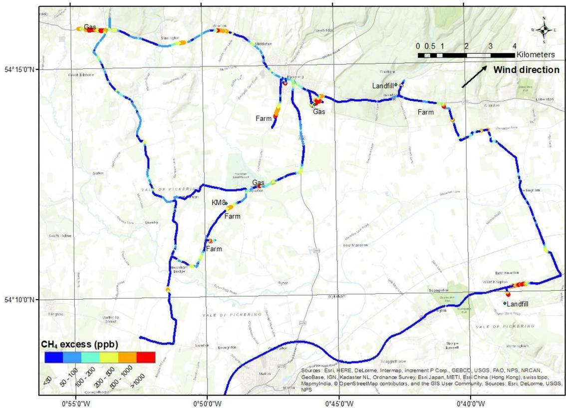
**Figure 65. Excess methane mole fraction above baseline for the Vale of Pickering survey area, 6 March 2018. The baseline for each survey day is defined as the average of the 2nd percentile of the data. © RHUL, 2018**
