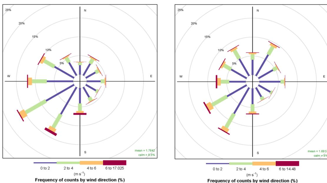
**Figure 33. Wind rose for the KM site, showing wind speed and direction statistics for: left: 1 Feb 2016 – 31 Jan 2017; right: 1 Feb 2017–31 Jan 2018. The radius defines the percentage of total time in each of 12 wind direction cones (30 degree span), while the colour scale (see colour legend) defines the wind speed. © University of Manchester, 2018.**
