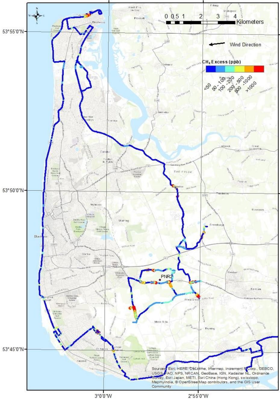
**Figure 48. Excess methane mole fraction above baseline for the Fylde survey area, 27 February 2018. The baseline for each survey day is defined as the 2nd percentile of the data. © RHUL, 2018**
