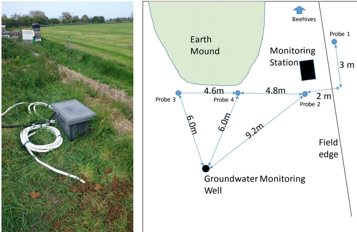
**Figure 106. Soil gas monitoring station appearance (left) and layout in 2017-18 (right)**
