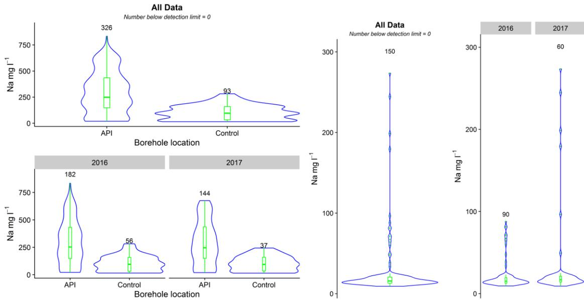
**Figure 14. Violin plots (box plots with kernel density estimation) for Na in samples collected between September 2015 and January 2018 left: groundwater; right: streams. API: area of potential impact**
