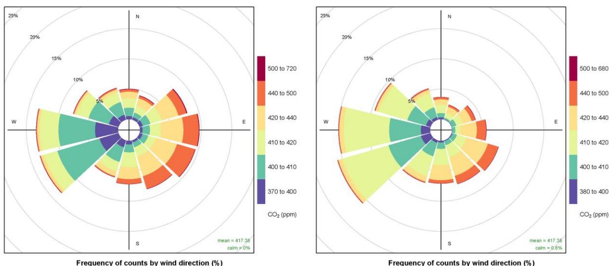
**Figure 36. Concentration (as per colour scale) wind roses for carbon dioxide (units of ppm), as measured at LP for the 2016-17 period (left panel) and 2017-18 period (right panel). © University of Manchester, 2018**
