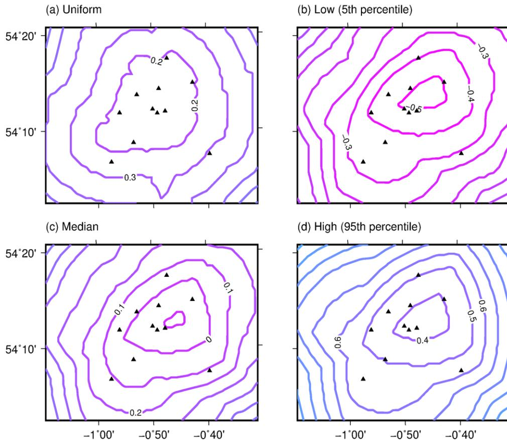
**Figure 26. Modelled detection capability using observed noise levels for each station in (a) uniform, (b) low, (c) median and (d) high noise conditions. A signal in excess of three times the noise level is required at five or more stations for an earthquake to be detected**
