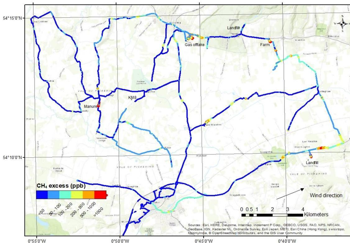
**Figure 64. Excess methane mole fraction above baseline for the Vale of Pickering survey area, 26 October 2017. The baseline for each survey day is defined as the average of the 2nd percentile of the data. © RHUL, 2018**
