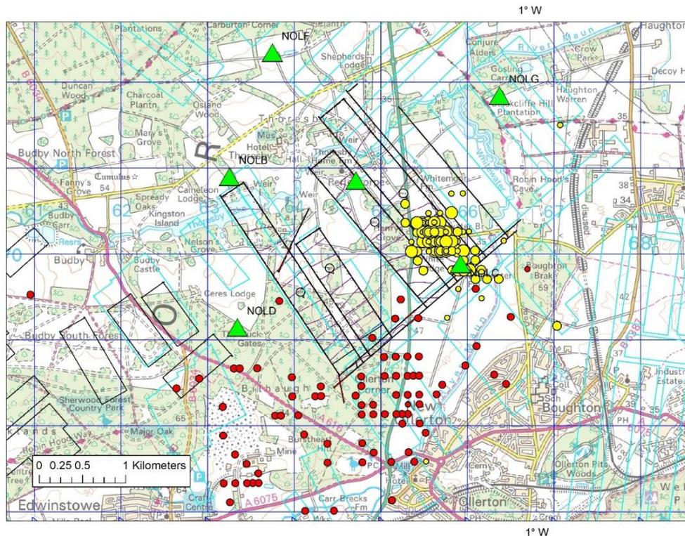
**Figure 30. Location calculated for earthquakes at Thoresby Colliery. The red dots are the locations using the national network only. The yellow dots are the locations also using the local network shown by the green triangles. The black rectangles are coal seams at 1 km depth. © Crown Copyright and/or database right, 2018. Licence number 100021290 EUL**
