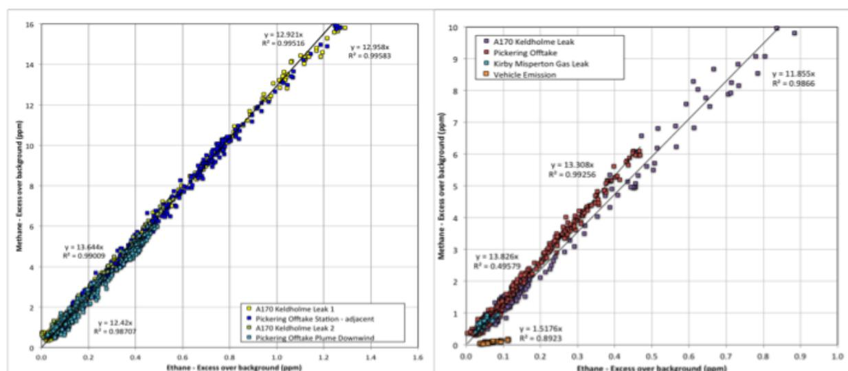
**Figure 67. Methane:ethane excess cross plot for fugitive gas emissions identified during the Vale of Pickering March 2018 mobile surveys. Left: 6<sup>th</sup>, Right: 7<sup>th</sup>. The multiplier of x is the ratio for the whole plume with CH<sub>4</sub> excess >0.5 ppm, except for the vehicle emission, which is >0.05 ppm. © RHUL, 2018**
