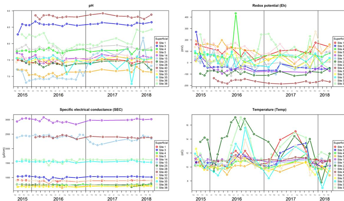
**Figure 2. Physico-chemical parameters monitored in groundwater from the Superficial aquifer**
