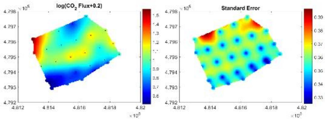
**Figure 114. Geostatistical prediction of log (CO<sub>2</sub> flux +0.2) with measurement locations denoted by black dots (left) and associated standard errors (right). Units are log(g/m<sup>2</sup>/d<sup>1</sup>)**
