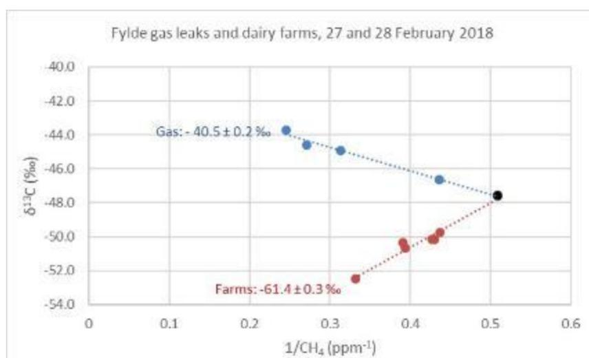
**Figure 45. Keeling plot identifying the isotopic source signatures of gas leak and dairy farm methane emissions in the Fylde for samples collected on 27th and 28th February 2018.**
