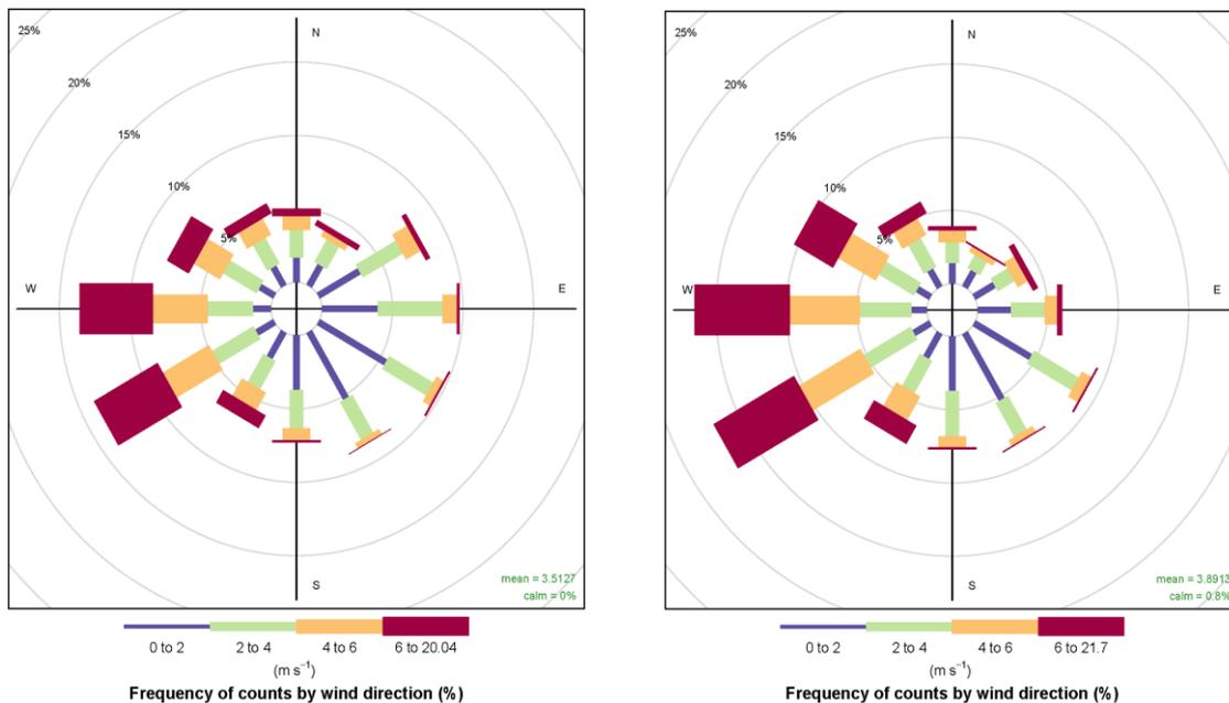
**Figure 32. Wind rose for the LP site, showing wind speed and direction statistics for: (left): 1 Feb 2016–31 Jan 2017; (right): 1 Feb 2017–31 Jan 2018. The radius defines the percentage of total time in each of 12 wind direction cones (30 degree span), while the colour scale (see colour legend) defines the wind speed. © University of Manchester, 2018**
