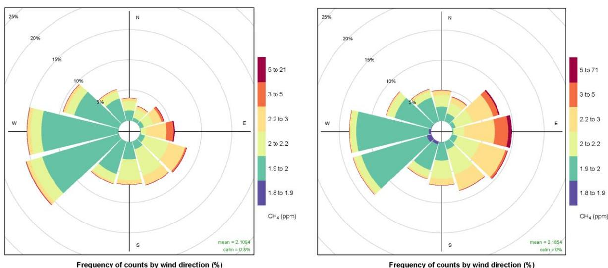
**Figure 35. Concentration (as per colour scale) wind roses for methane (units of ppm), as measured at LP for the 2016-17 period (left panel) and 2017-18 period (right panel). © University of Manchester, 2018.**
