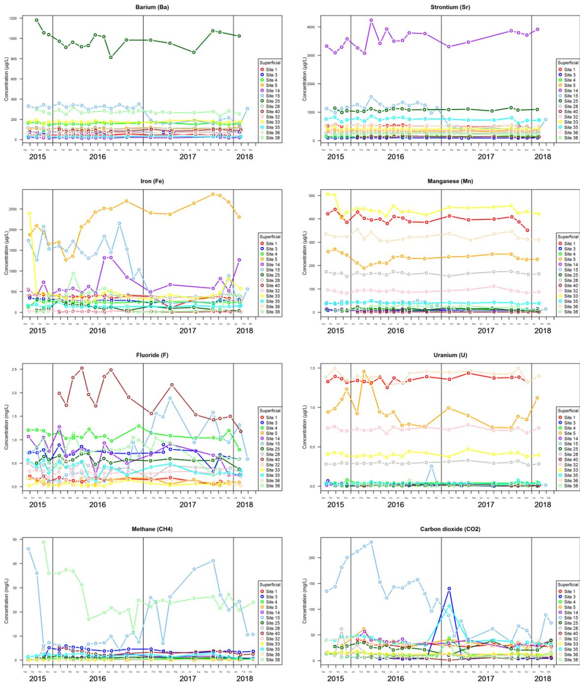
**Figure 4. Data for selected minor ions and dissolved gases in groundwater from the Superficial aquifer**
