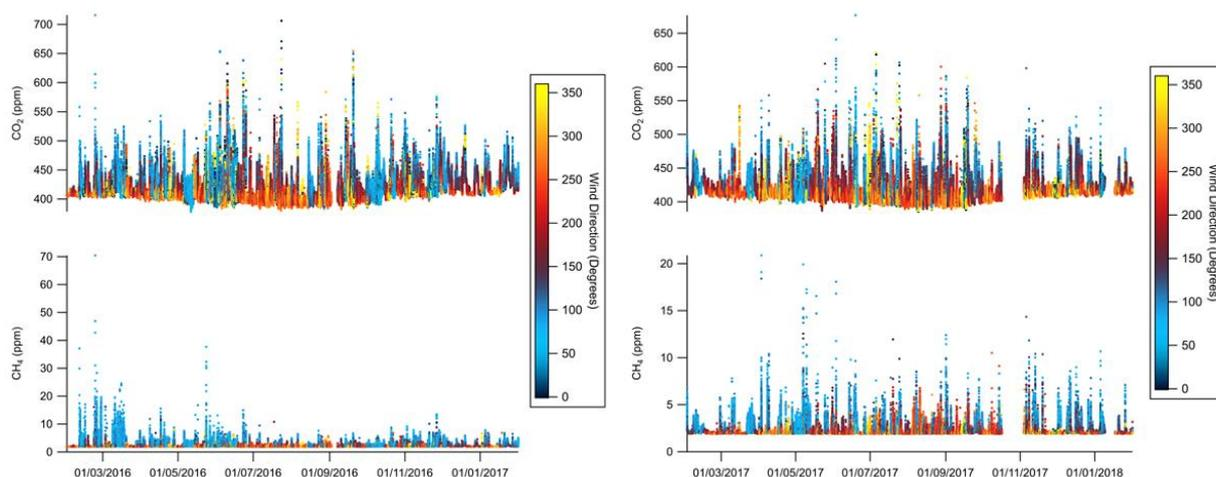
**Figure 37. Concentrations (as per colour scale) in air as a function of time (x-axis) and wind direction (colour-coding) for carbon dioxide (top panels), and methane (bottom panels) as measured at LP for the 2016-17 baseline period (left panel) and 2017-18 period (right panel). © University of Manchester, 2018**
