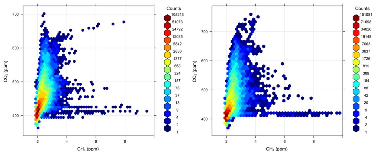
**Figure 55. Coincident CO<sub>2</sub> and CH<sub>4</sub> concentrations measured at KM for the 2016-17 period (left panel) and 2017-18 period (right panel). Colours indicate the frequency density of sampling (number of coincident measurements). Note: one count refers to a one-minute period of data. © University of Manchester, 2018**
