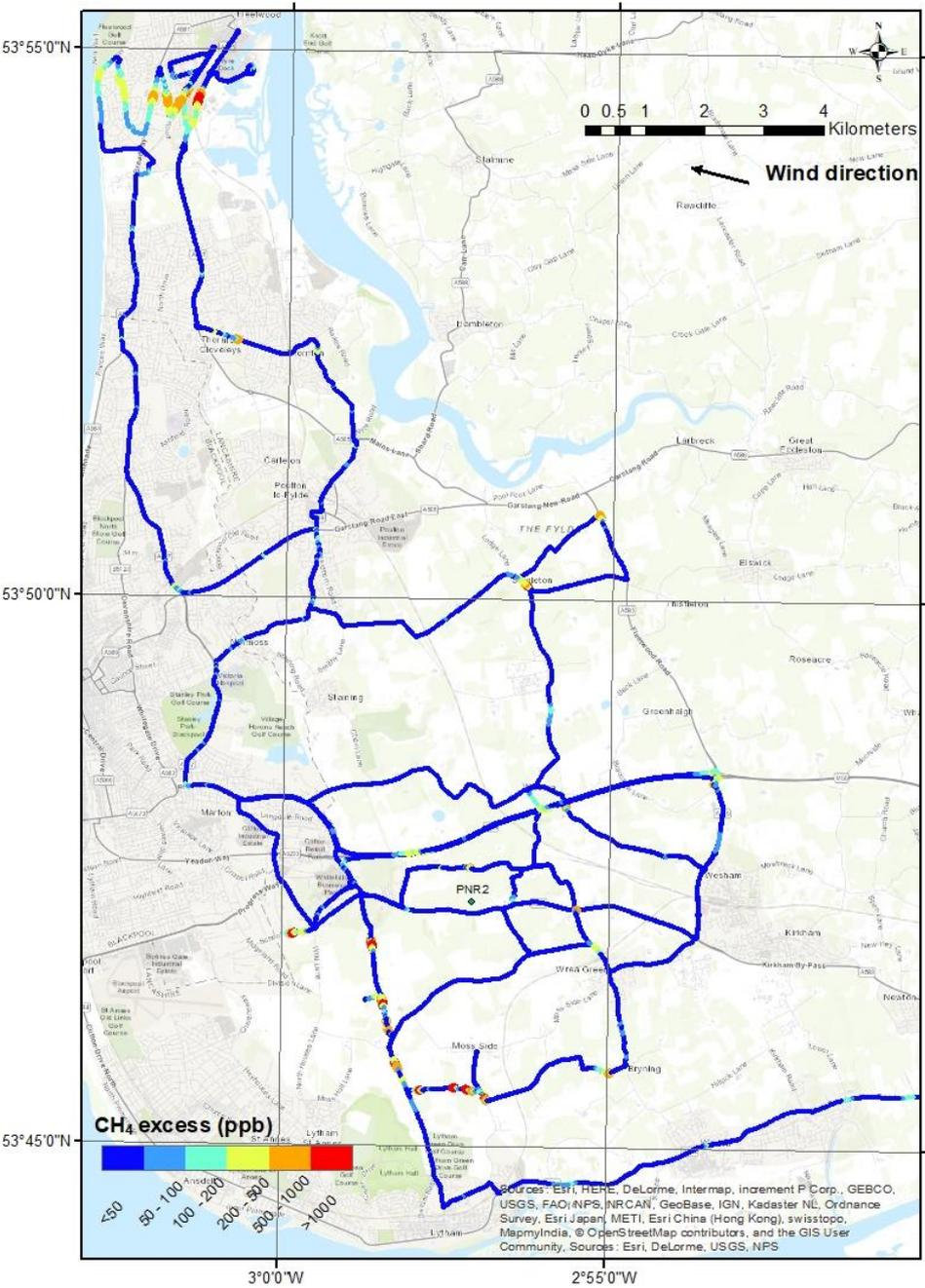
**Figure 47. Excess methane mole fraction above baseline for the Fylde survey area, 27 June 2017. The baseline for each survey day is defined as the 2nd percentile of the data. © RHUL, 2018**
