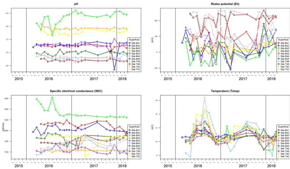
**Figure 5. Physico-chemical parameters in groundwater from the BGS boreholes in the Superficial aquifer**
