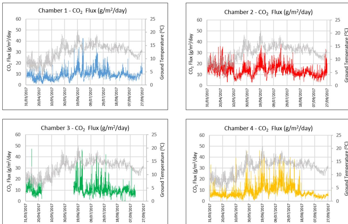
**Figure 102. Individual continuous time series plots of CO<sub>2</sub> flux from chambers 1, 2, 3 and 4, along with ground temperature**
