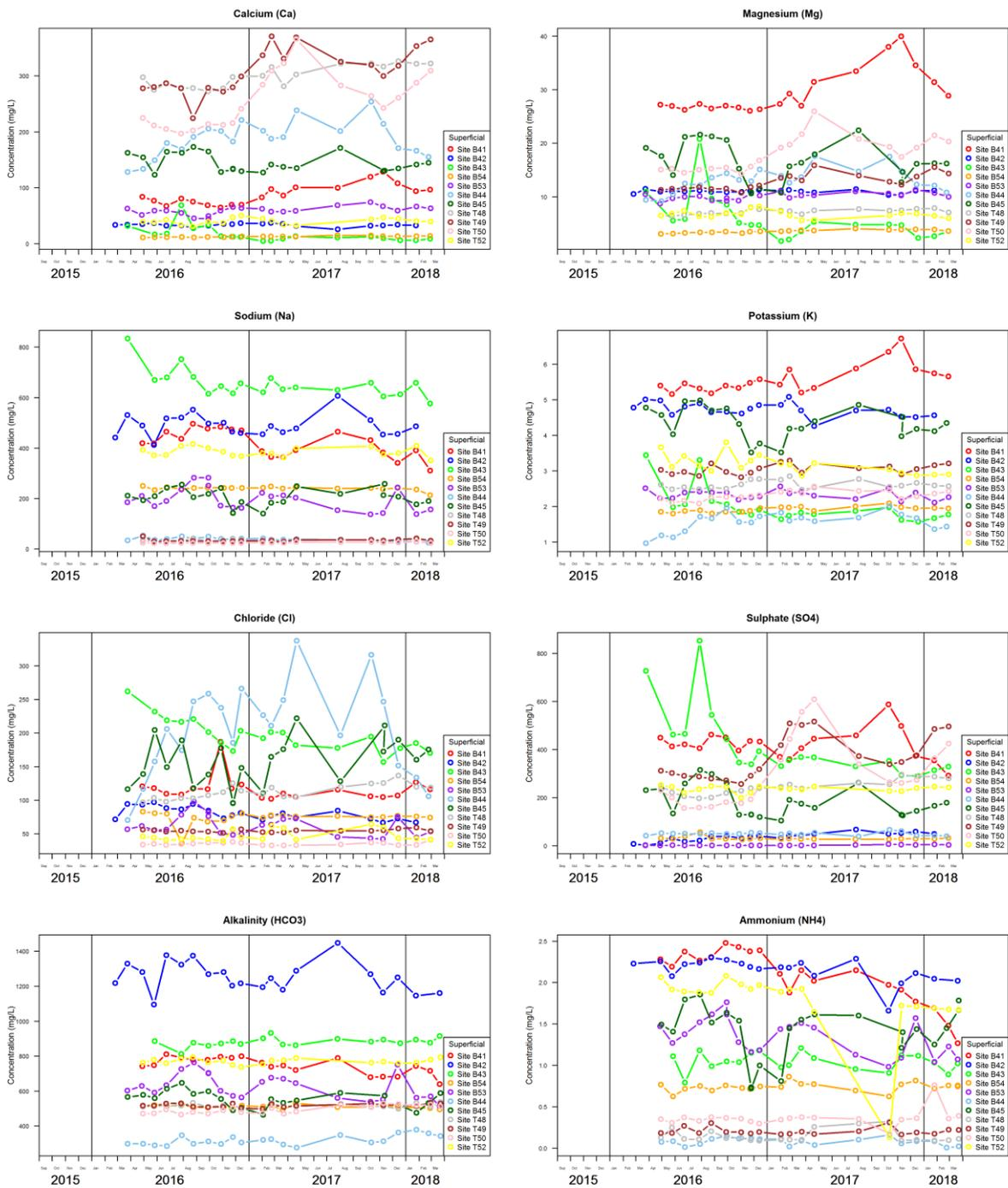
**Figure 6. Major ions and ammonium in groundwater from BGS boreholes in the Superficial aquifer**
