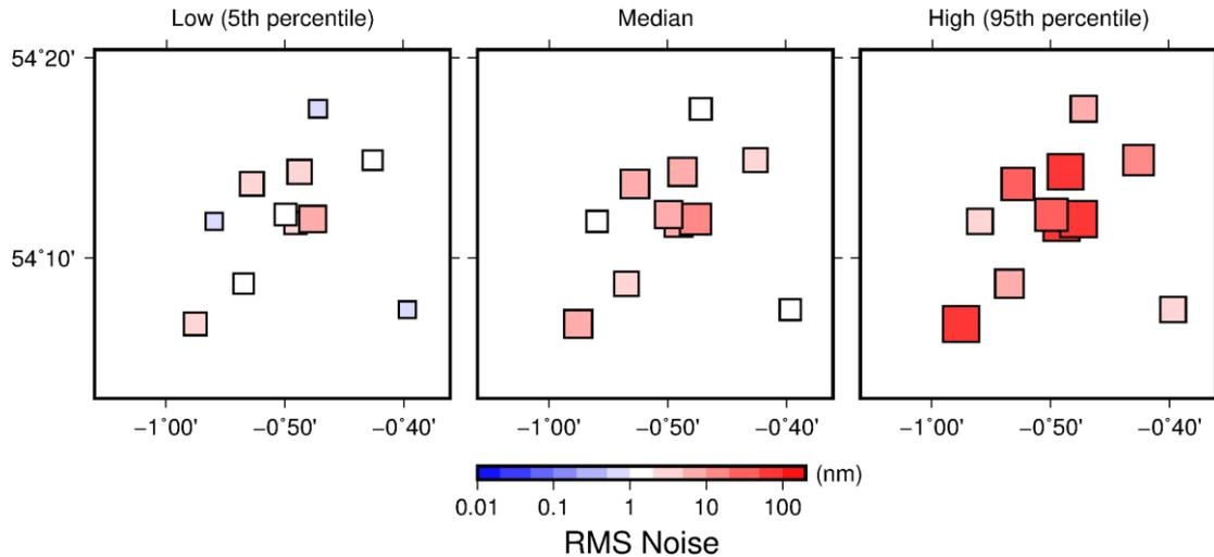
**Figure 25. Observed RMS noise levels determined from power spectral density estimates for each day over the time period 01/04/2016 to 31/03/2017**
