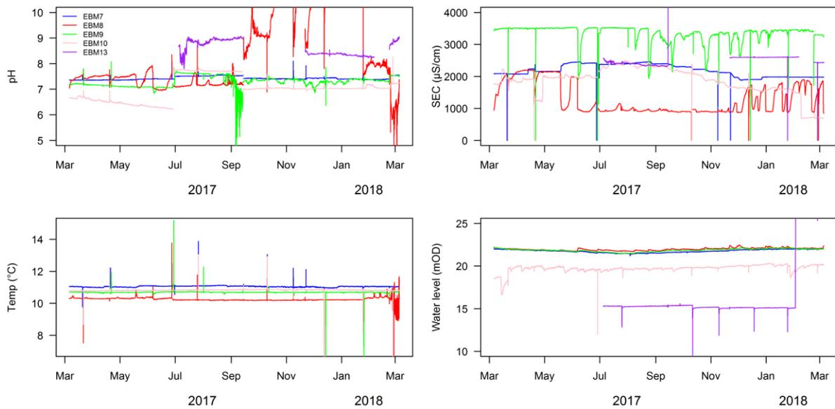
**Figure 17. Real-time monitoring data (pH, SEC, temperature and groundwater level) from five sondes within boreholes in the BGS groundwater monitoring network**
