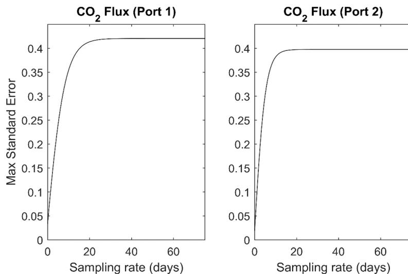
**Figure 118. Standard errors for temporal log (CO<sub>2</sub> flux +0.2) predictions at the time midway between two measurements as a function of time between measurements**
