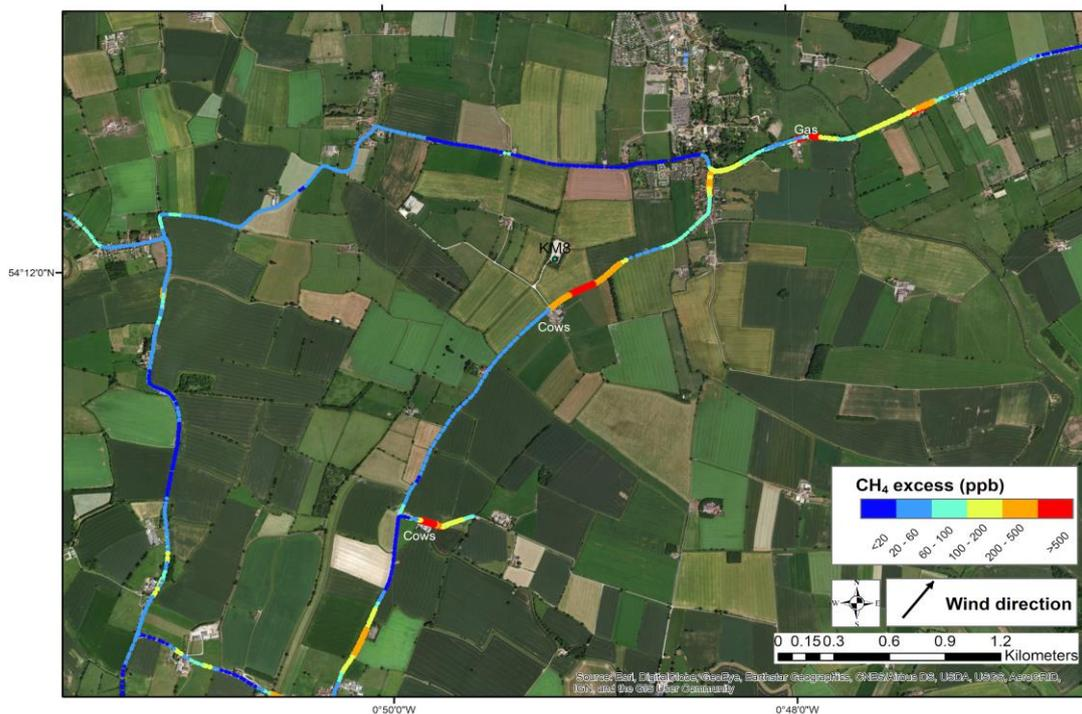
**Figure 66. Excess methane mole fraction above baseline for the area around the KM8 well, Vale of Pickering, 06 March 2018. The baseline for each survey day is defined as the average of the 2nd percentile of the data. Note methane elevations from dairy farms to the S and SSW and a gas leak to the ENE of the KM8 site. (Basemap imagery sources: Esri, DigitalGlobe, GeoEye, Earthstar Geographics, CNES/Airbus DS, USDA, USGS, AeroGRID, IGN, and the GIS User Community). © RHUL, 2018**
