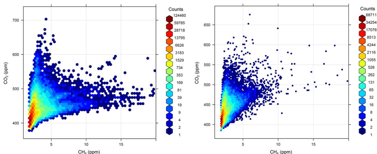
**Figure 38. Coincident  $\text{CO}_2$  and  $\text{CH}_4$  concentrations measured at LP for the 2016-17 period (left panel) and 2017-18 period (right panel). Colours indicate the frequency density of sampling (number of coincident measurements). N.B. One count refers to a one-minute period of data. © University of Manchester, 2018**
