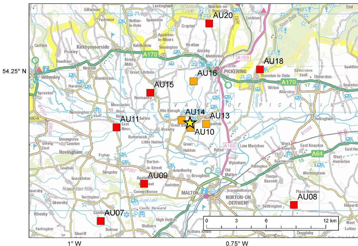
**Figure 20. Ordnance Survey map of the Vale of Pickering. Red squares show the surface sensors and the orange squares show the locations of the borehole sensors. There are also surface sensors co-located with some of the borehole sensors. The yellow star shows the location of the drill site. © Crown Copyright and/or database right, 2018. Licence number 100021290 EUL**
