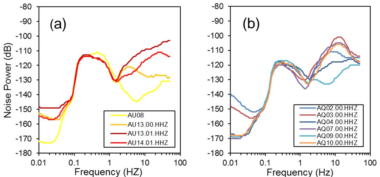
**Figure 24. Comparison of the median noise levels at the selected stations in the (a) Vale of Pickering and (b) Fylde networks**
