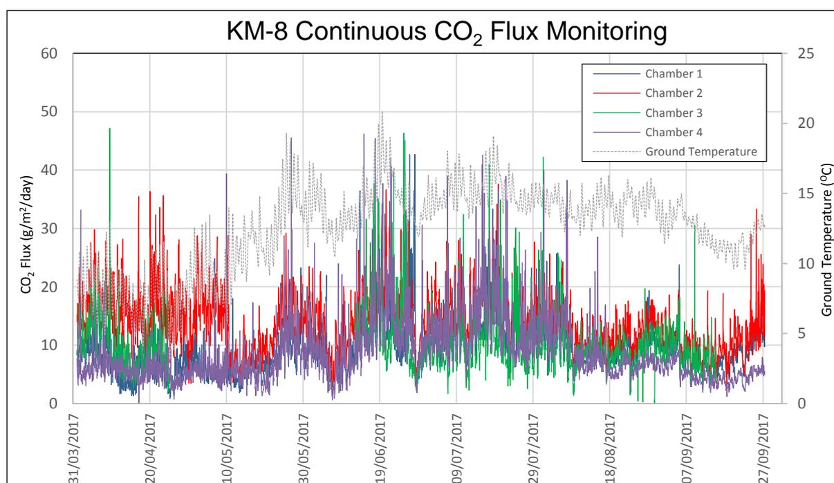
**Figure 101. Continuous time series plot of CO<sub>2</sub> flux from chambers 1, 2, 3 and 4, along with ground temperature**
