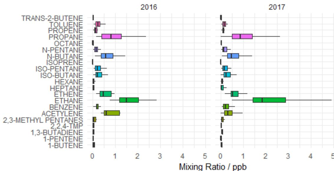
**Figure 87. Box and whisker plot of NMHCs measured at LP in 2016 and 2017.**
