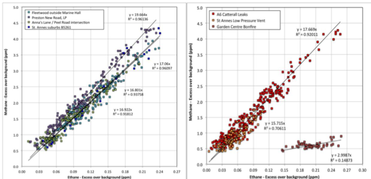
**Figure 50. Methane:ethane excess cross plots for fugitive gas emissions identified during the Fylde February 2018 mobile survey. Left: 27<sup>th</sup>, Right: 28<sup>th</sup>. The multiplier of x is the ratio for the whole plume with CH<sub>4</sub> excess >0.5 ppm. © RHUL, 2018**
