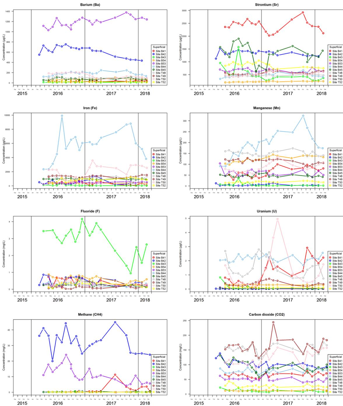
**Figure 7. Minor ions and dissolved gases in groundwater from BGS boreholes in the Superficial aquifer**
