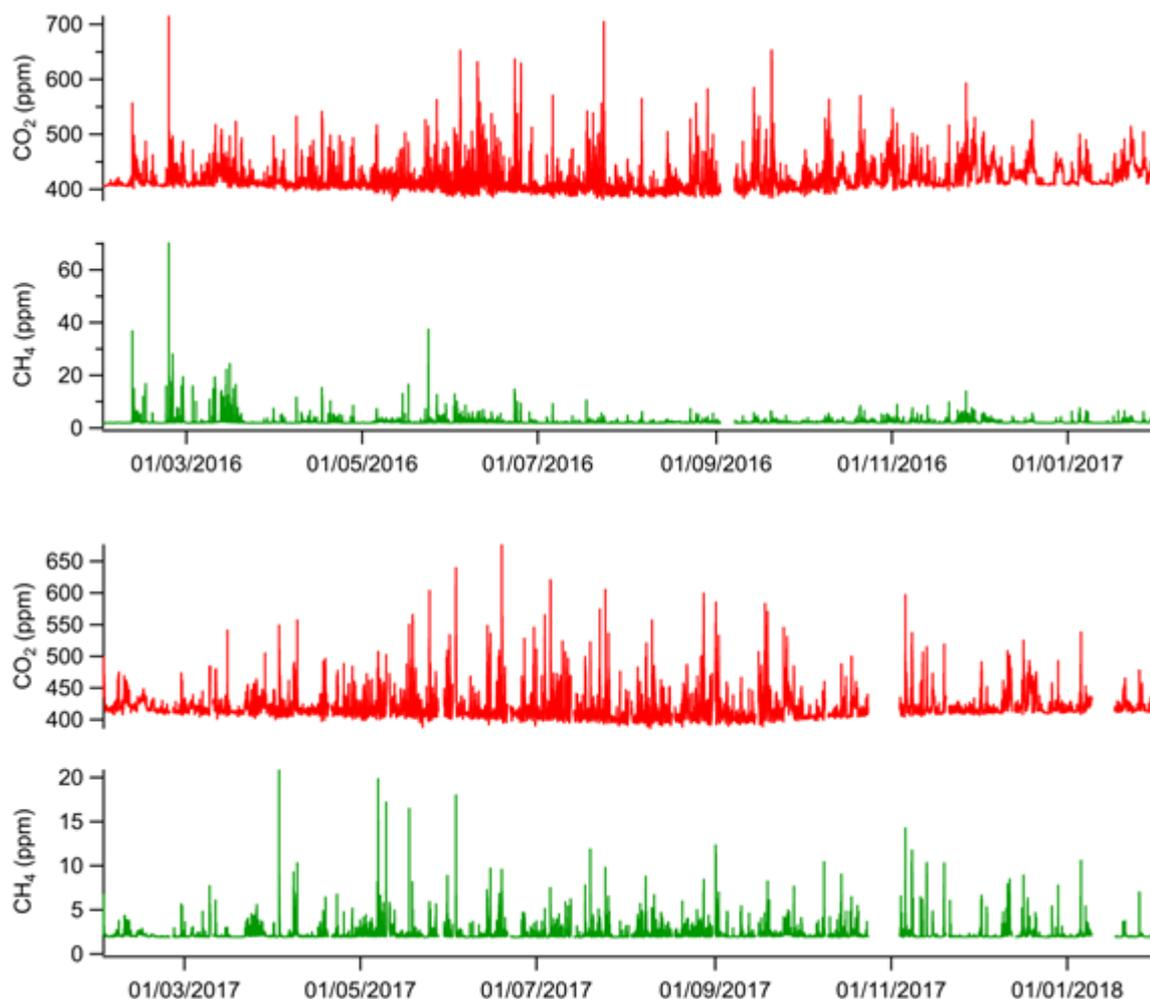
**Figure 34. Time series of carbon dioxide (red) and methane (green) in units of ppm measured at LP between: 1 Feb 2016 and 31 Jan 2017 (top panels); 1 Feb 2017-31 Jan 2018 (bottom panels). © University of Manchester, 2018.**
