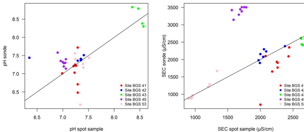
**Figure 18. Comparison of pH and SEC values for groundwater collected during the monitoring rounds with values determined by sondes in real-time (1:1 lines also shown)**
