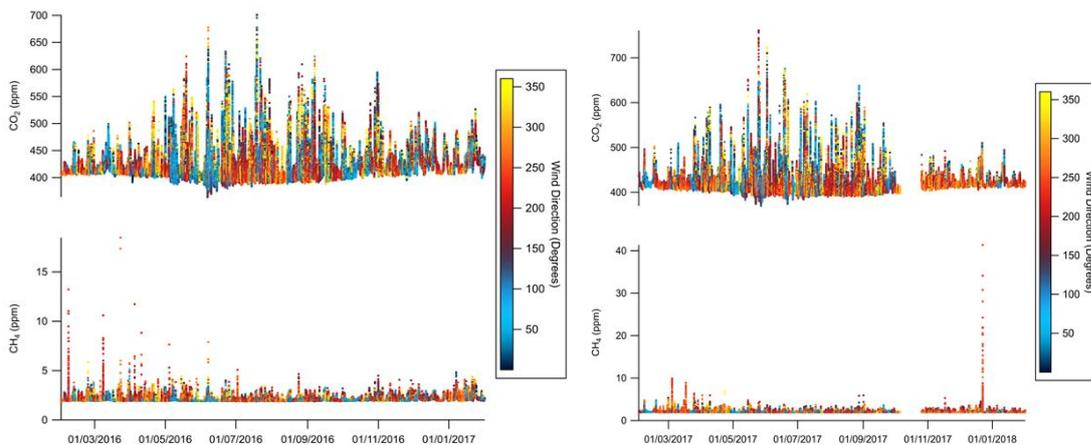
**Figure 54.** Concentrations (as per colour scale) in air as a function of time (x-axis) and wind direction (colour-coding) for carbon dioxide (top panels), and methane (bottom panels) as measured at KM for the 2016–17 baseline period (left panel) and 2017-18 period (right panel). © University of Manchester, 2018
