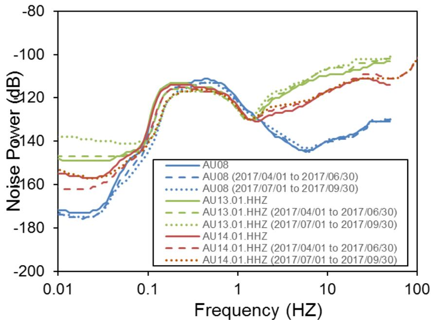
**Figure 23. Median noise levels at all stations in the Vale of Pickering network as a function of frequency. AU10, AU13.00, AU14.00 and AU16 are borehole sensors. All other sensors are at the surface**
