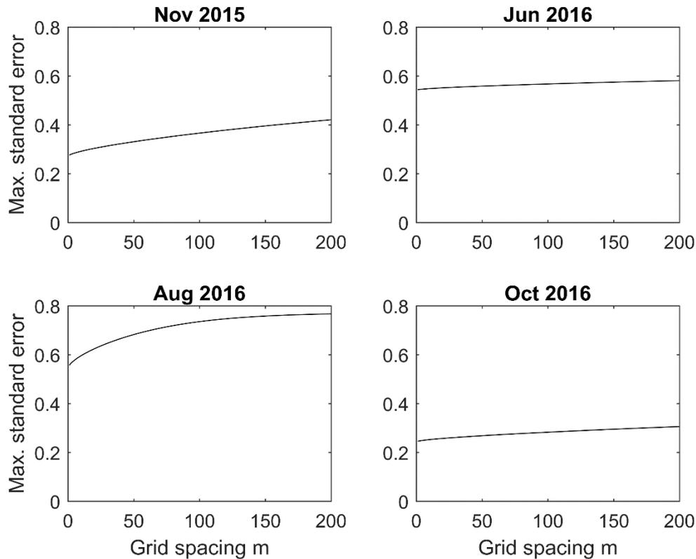
**Figure 116. Standard errors for spatial log (CO<sub>2</sub> flux +0.2) predictions at the centre of 81-point regular square grids of different sizes**
