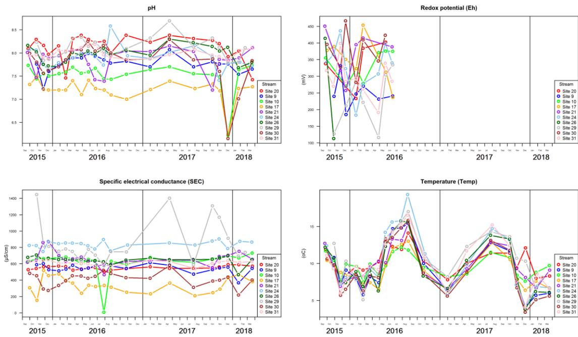
**Figure 11. Variation in physico-chemical compositions of streams in the Vale of Pickering (Note: redox potential (Eh) only measured for a short period to cross-check electrode performance and confirm oxidising condition)**
