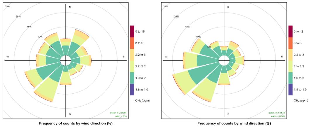
**Figure 52.** Concentration (as per colour scale) wind rose for methane as measured at KM in the 2016–17 baseline period (left) and 2017–18 period (right). Radial extent contours define 2% frequency intervals. © University of Manchester, 2018
