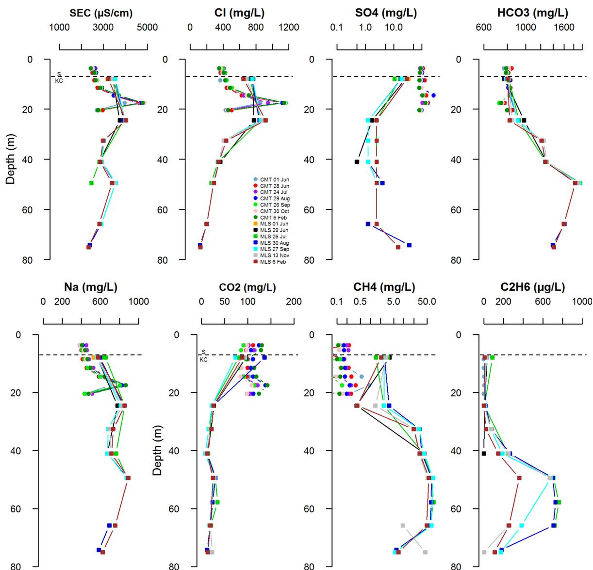
**Figure 19.** Profiles of selected analytes from a multi-level sampler array sited some 2 km east of KM8; CMT: Solinst Continuous Multichannel Tubing; MLS: Solinst Waterloo multi-level sampler; S: Superficial (Quaternary) aquifer; KC: Kimmeridge Clay
