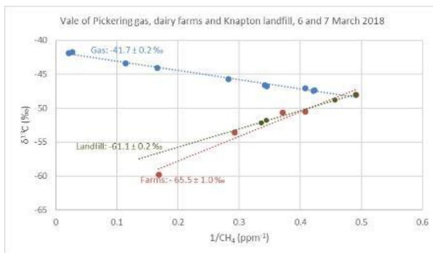
**Figure 62. Keeling plot to identify methane  $\delta^{13}\text{C}$  signature of gas leaks, dairy farms and Knapton landfill site in the Vale of Pickering, 6-7 March 2018. © RHUL, 2018**
