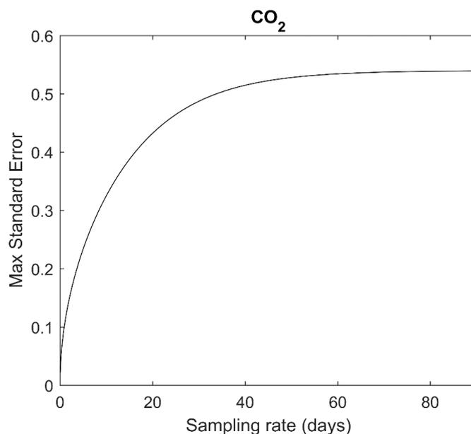
**Figure 119. Standard errors for temporal log (CO<sub>2</sub> concentration +0.2) predictions at the time midway between two measurements as a function of time between measurements**
