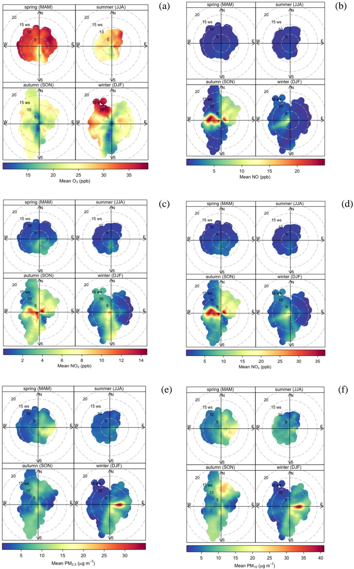
**Figure 74. Polar plots for KM for concentrations of (a)  $O_3$ , (b) NO, (c)  $NO_2$ , (d)  $NO_x$ , (e)  $PM_{2.5}$ , (f)  $PM_{10}$ . © University of York, 2018**
