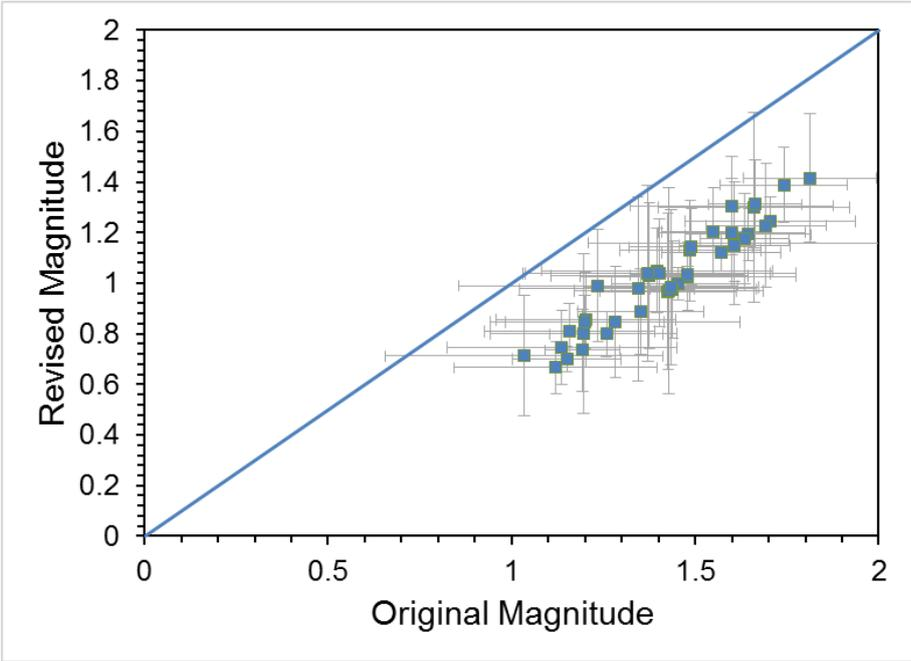
**Figure 31. Local magnitudes for Newbridge Quarry events calculated with the Hutton and Boore (1987) scale and a revised scale to correct for overestimation of magnitude at short epicentral distances (Luckett et al, 2018). Error bars show standard deviation in individual station measurements**
