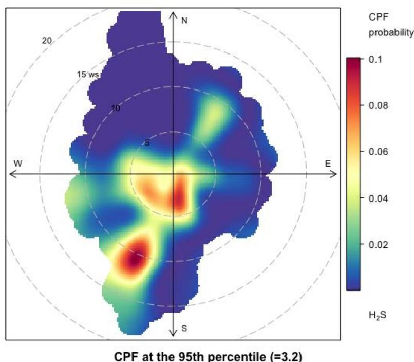
**Figure 80. Polar plot of H<sub>2</sub>S concentrations at KM8 based on the CPF function.**
