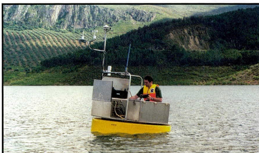
Figure 57. Testing the Automatic Water Quality Monitoring Station during installation at Embalse de Iznajar (Spain).
