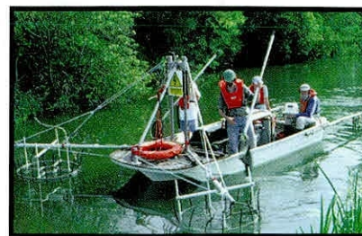
Figure 44. Electro-fishing on the Great Ouse using a boom boat.
