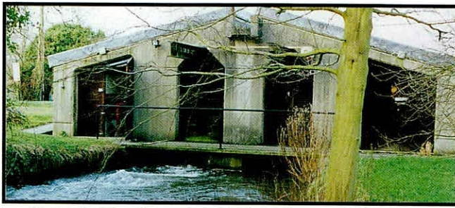
Figure 27. Fluvarium at the IFE, River Laboratory, used to measure nutrient fluxes in polluted and unpolluted river sediments; river water from the R. Frome is used to maintain the bed-sediment temperature as close to natural conditions as possible.
