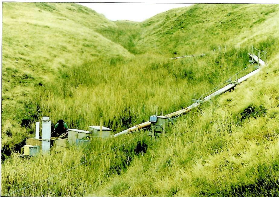
Plate 32. The Cerrig yr Wyn field site, showing the diversion of inflowing waters through a system of pipes in order to simulate drought in the lower wetland. The intact control wetland is visible in the background
