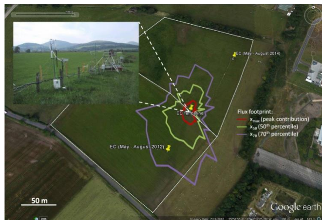
Fig. 1: Experimental field sites at Easter Bush, Scotland. The EC system comprises a LI-COR 7000 closed-path analyser and a Gill Instruments Windmaster Pro ultrasonic anemometer mounted atop a 2.5 m mast located along the fence line separating the fields. The locations of the temporary EC systems used for the 2012 and 2014 ploughing events are marked EC 2012 and EC 2014.
