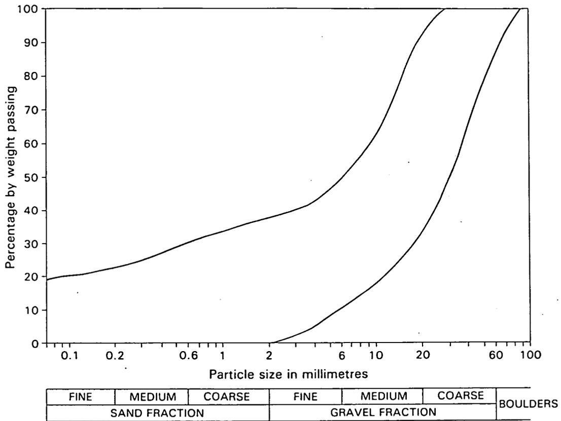
Figure 6. Grading 'envelope' for river terrace deposit gravel (170 samples)
