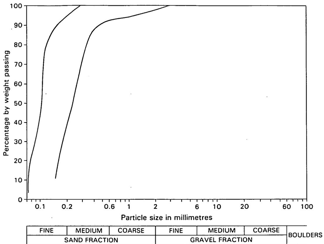
Figure 8. Grading 'envelope' for Whitecliff Sand (20 samples)
