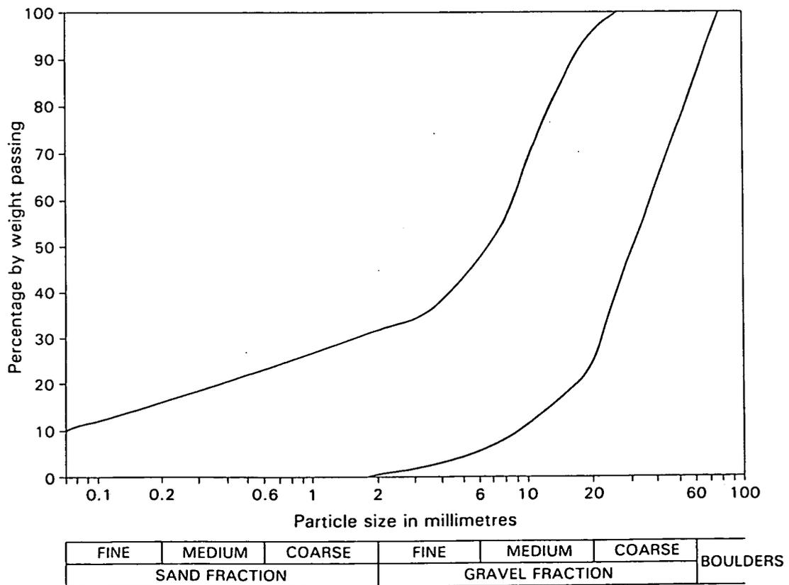
Figure 7. Grading 'envelope' for alluvium (45 samples)
