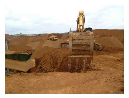
**Figure 2.** Marlstone Rock Formation ironstone being worked for crushed rock aggregate at Wroxton Fields Quarry near Banbury, Peter Bennie Ltd.
